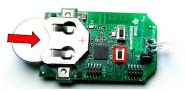
Figure 1. Insert Battery
