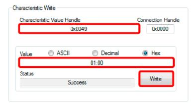
If a button on the CC2541 Keyfob is now pushed, notifications are sent, and can be monitored in the BTool log window.
