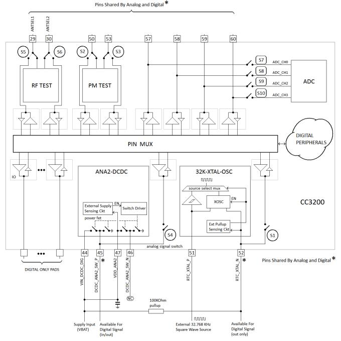
Board level configuration required to use Pin 45 and Pin 52 for digital signals
