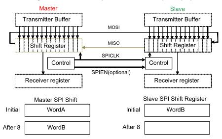
Figure 8-2. SPI Full Duplex Transmission (Example)
