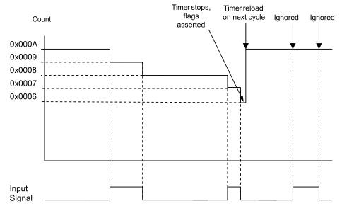
Figure 9-2. Input Edge-Count Mode Example, Counting Down
