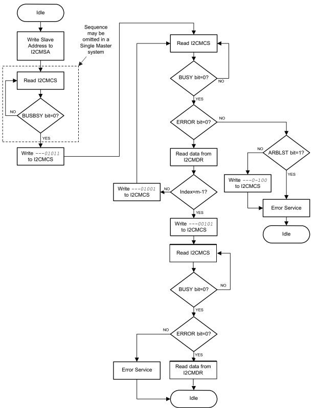
Figure 7-10. Master RECEIVE of Multiple Data Bytes
