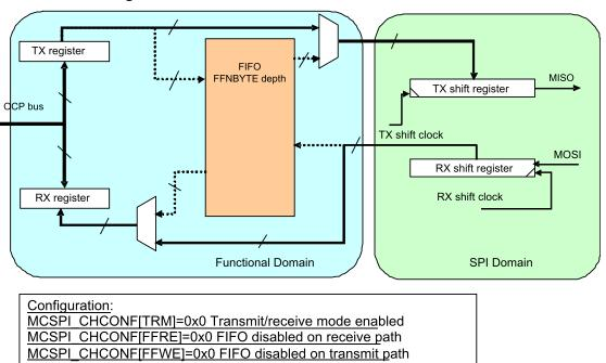
Figure 8-6. Transmit/Receive Mode With no FIFO Used
