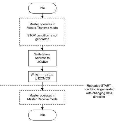
Figure 7-11. Master RECEIVE with Repeated START after Master TRANSMIT
