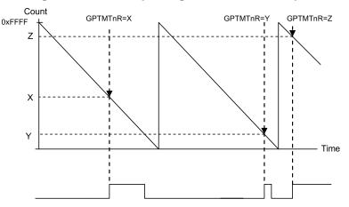
Figure 9-3. 16-Bit Input Edge-Time Mode Example
