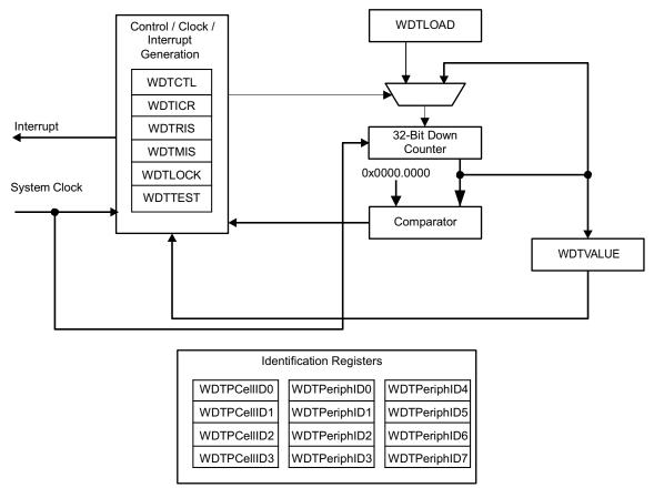
Figure 10-1. WDT Module Block Diagram
