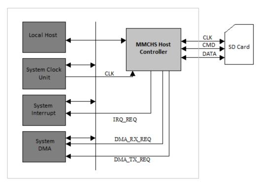
Figure 11-1. SDHost Controller Interface Block Diagram
