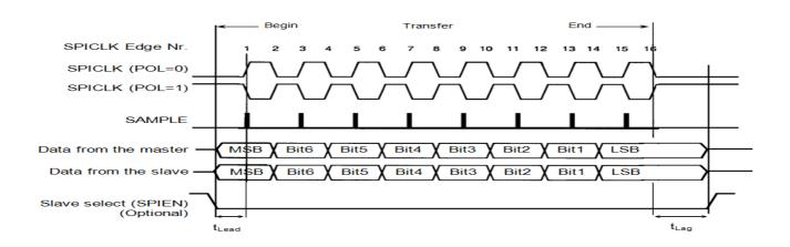
Figure 8-3. Full Duplex Single Transfer Format with PHA = 0
