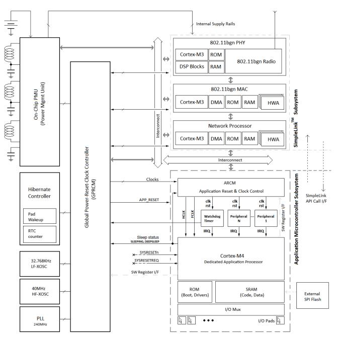
Figure 15-3. Power Management Control Architecture in CC3200
