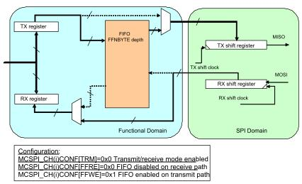
Figure 8-8. Transmit/Receive Mode With Only Transmit FIFO Used
