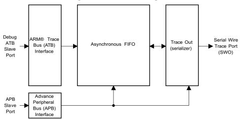
Figure 2-2. TPIU Block Diagram
