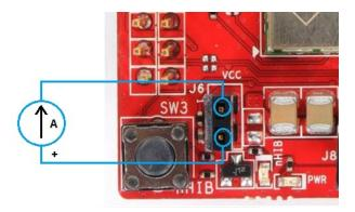
**Figure 9. Low Current Measurement**
