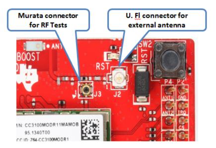
Figure 11. Connectors on the Board
