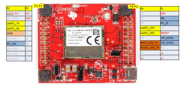
Figure 4. Signal Assignments
