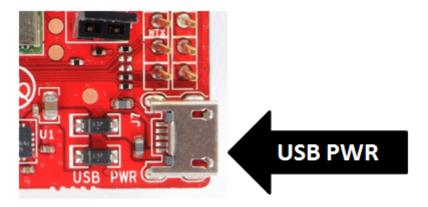
Figure 6. Feed USB on the BoosterPack (if the LaunchPad Cannot Source 5 V on 20-Pin Connector)
