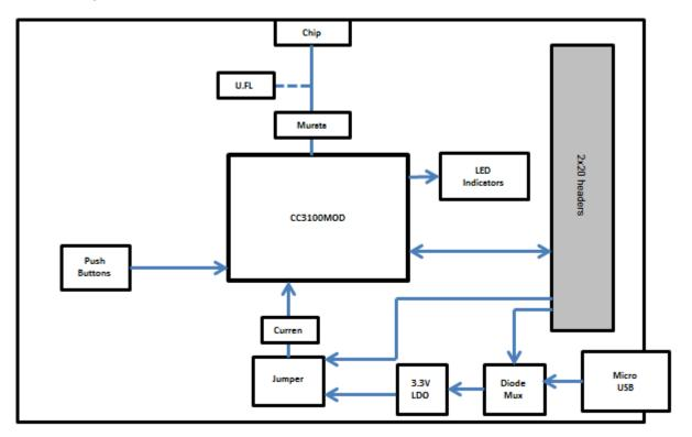
Figure 3. CC3100MODBOOST Block Diagram
