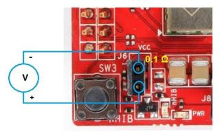
Figure 10. Active Current Measurement
