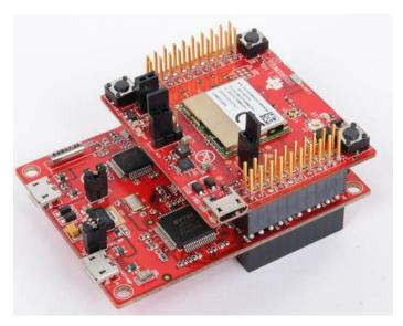
Figure 15. The CC3100BOOST Connected to the EMUBOOST
