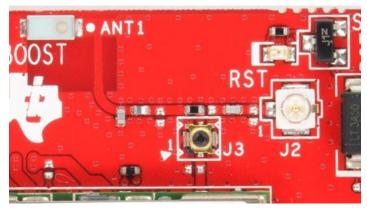
Figure 12. Resistor Switch for Radiated versus Conducted Tests
