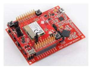
Figure 16. CC3100MODBOOST Connected to MSP430F5529 LaunchPad
