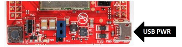
Figure 17. Jumper Settings When Used With LaunchPad
