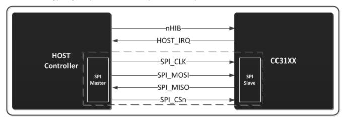
Figure D-1. Basic SPI Configuration
