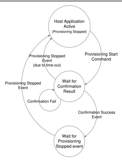
Figure 16-2. The Provisioning Process
