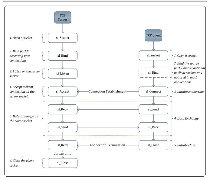
Figure 6-1. TCP Socket Flow
