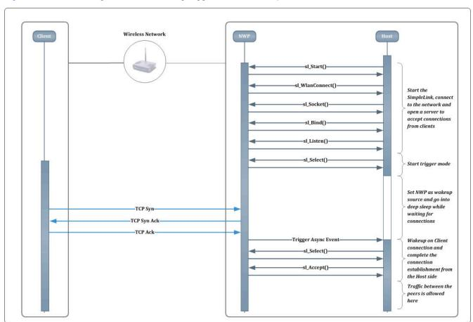
Figure 6-4. Trigger Mode Flow
