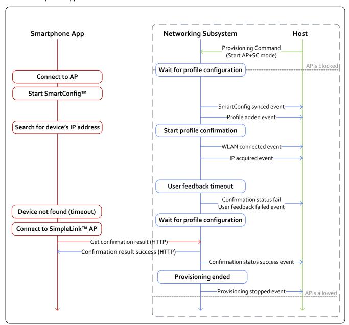
Figure 16-5. Successful SmartConfig Provisioning With AP Fallback
