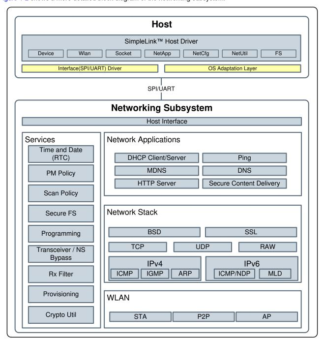
Figure 1-2. Networking Subsystem Block Diagram
