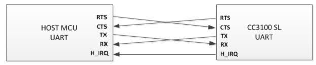
Figure D-12. Typical 5-Wire UART Configuration
