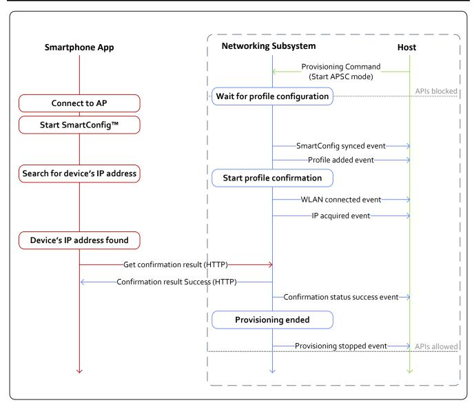
Figure 16-3. Successful SmartConfig Provisioning
