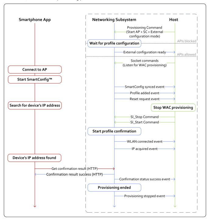
Figure 16-9. Successful SmartConfig Provisioning While External Configuration Enabled
