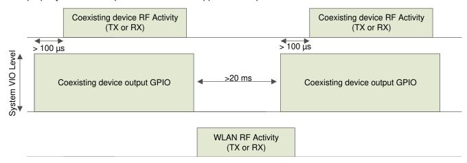
Figure 4-3. Coexistence Mechanism
