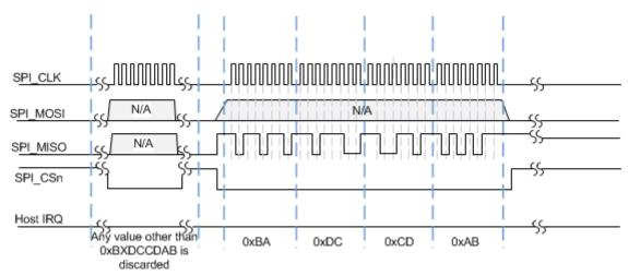
Figure D-7. CC3100 Device to Host Synchronization Word
