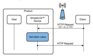
Figure 9-3. Reading Configuration
