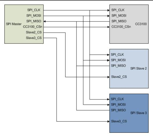
Figure D-4. Shared SPI Block Diagram
