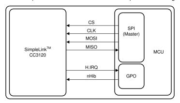
Figure 3-1. Typical CC31xx Setup (SPI)
