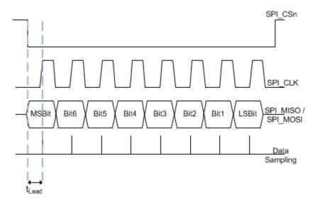
Figure D-3. SPI Mode 0 Detailed Timings
