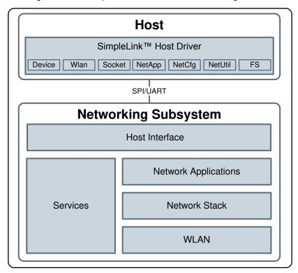
Figure 1-1. SimpleLink™ Wi-Fi® Solution Block Diagram
