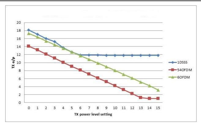
Figure 4-1. Tx Output Power vs Tx Power Settings
