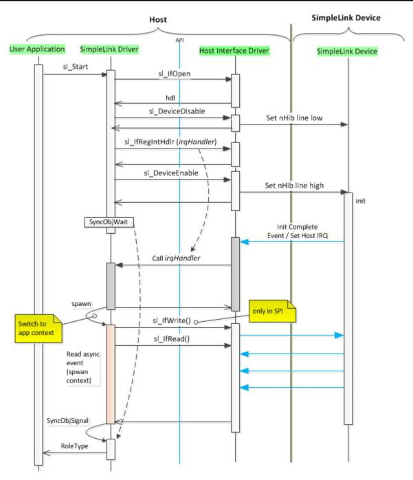
Figure D-5. SPI Initialization Flow
