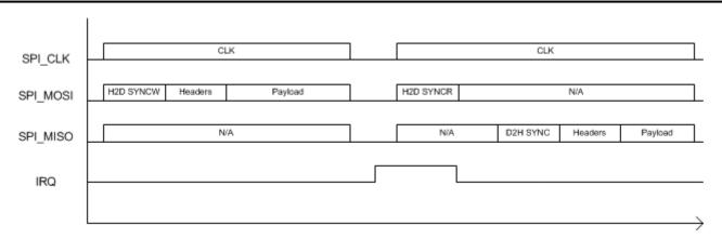
Figure D-8. CC31XX SPI Host Command Flow
