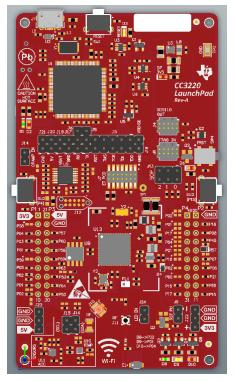
Figure 1. CC3220 SimpleLink Wi-Fi LaunchPad Development Kit
