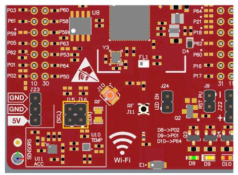
Figure 10. I<sup>2</sup>C Bus Connections
