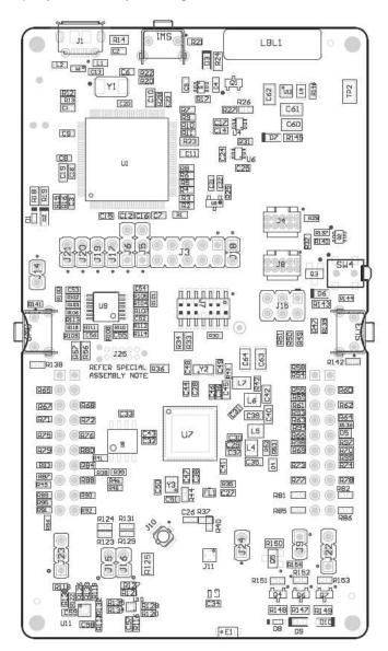
Figure 23. CC3220x LaunchPad Kit Top-Layer Assembly Drawing
