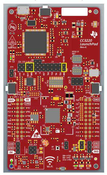
Figure 16. Powering From USB Jumper Settings
