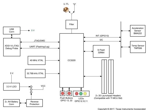
Figure 4. CC3220 Block Diagram
