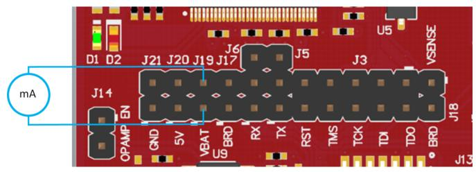
Figure 19. Low-Current Measurement (<1 mA)
