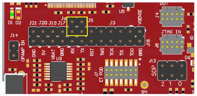
Figure 13. UART Routed to USB COM Port
