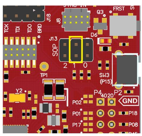
Figure 12. SOP Jumpers (Default Setting Shown)
