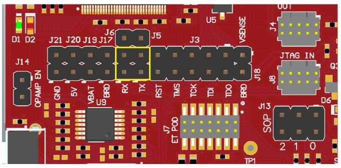
Figure 14. UART Routed to 20-Pin Header Connector
