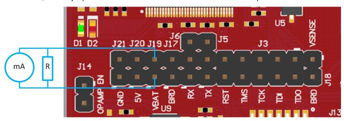
Figure 20. Active Power Measurements (>1 mA)
