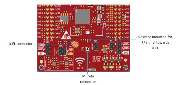
Figure 22. Board Modified for External Antenna Connections
