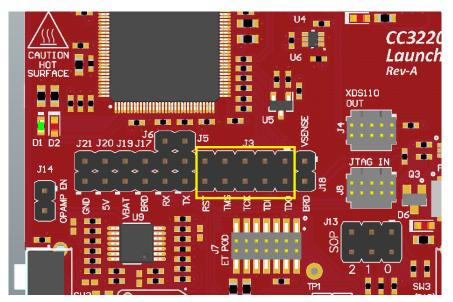
Figure 7. Default Jumper Configuration for JTAG Lines
