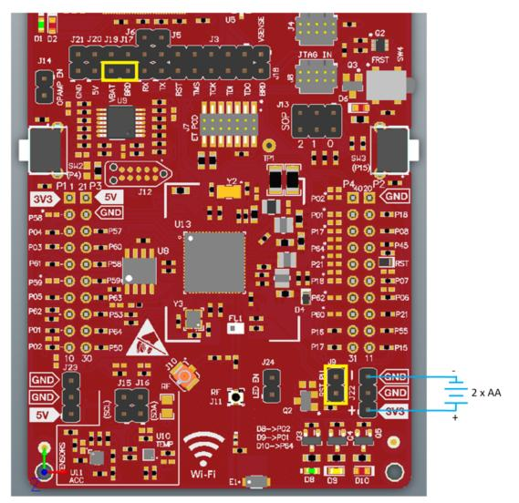
Figure 17. Powering the CC3220LP From Battery
