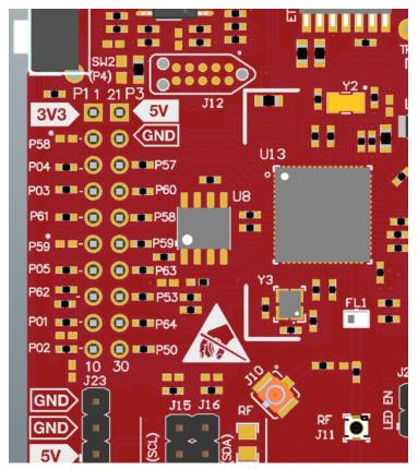
Figure 5. Pin 1 Marking on CC3220LP (3V3 Tag)
