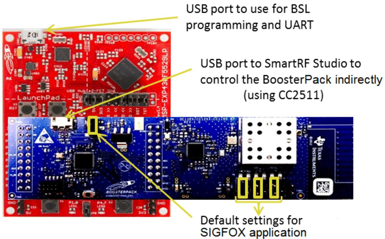
**Figure 1-2. LaunchPad and BoosterPack Board Settings for ETSI/ARIB SIGFOX Applications**
