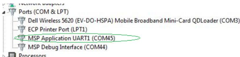
7. Set up the serial port that is identified by MSP Application UART1 (see Figure 1-5).
