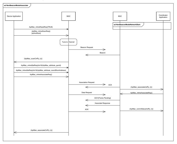
Figure 4-10. Nonbeacon Mode Device Association Sequence
