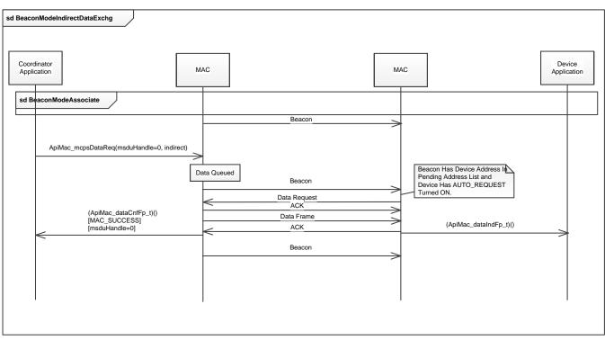
Figure 4-4. Beacon Mode Indirect Data Exchange Sequence
