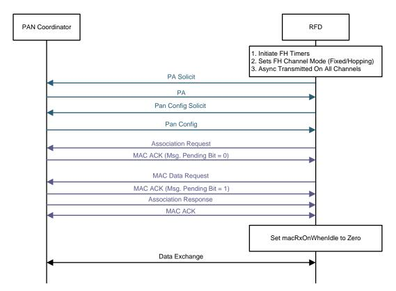
Figure 4-21. Joining Procedure for a Nonsleepy Frequency-Hopping Device
