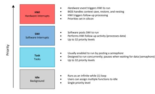
Figure 3-1. RTOS Execution Threads
