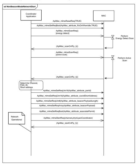
Figure 4-9. Nonbeacon Mode Network Start-Up Sequence
