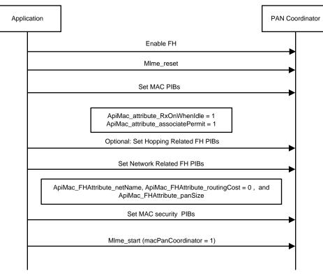
Figure 4-18. Start-Up Sequence of PAN Coordinator
