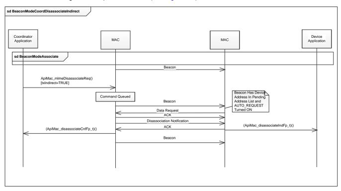
Figure 4-6. Beacon Mode Coordinator Initiated Indirect Disassociation Sequence
