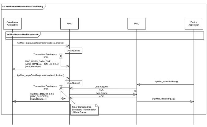
Figure 4-12. Nonbeacon Mode Indirect Data Exchange Sequence
