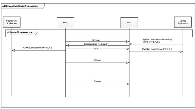
Figure 4-8. Beacon Mode Device-Initiated Disassociation Sequence
