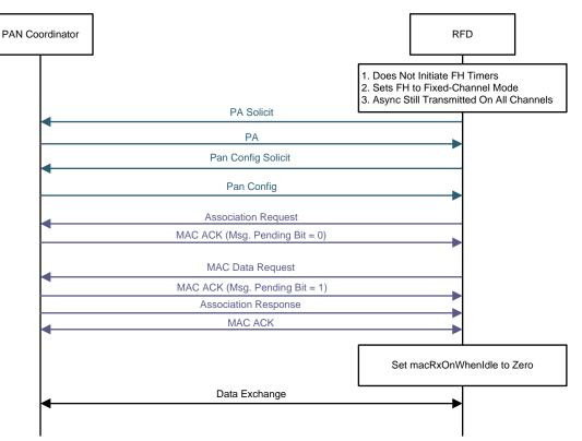
Figure 4-20. Joining Procedure for a Sleepy Frequency-Hopping Device
