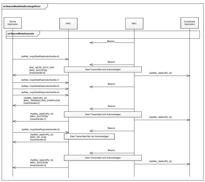
Figure 4-3. Beacon Mode Direct Data Exchange Sequence
