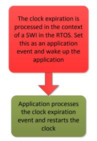
Figure 3-4. Clock Expiration Flow Diagram
