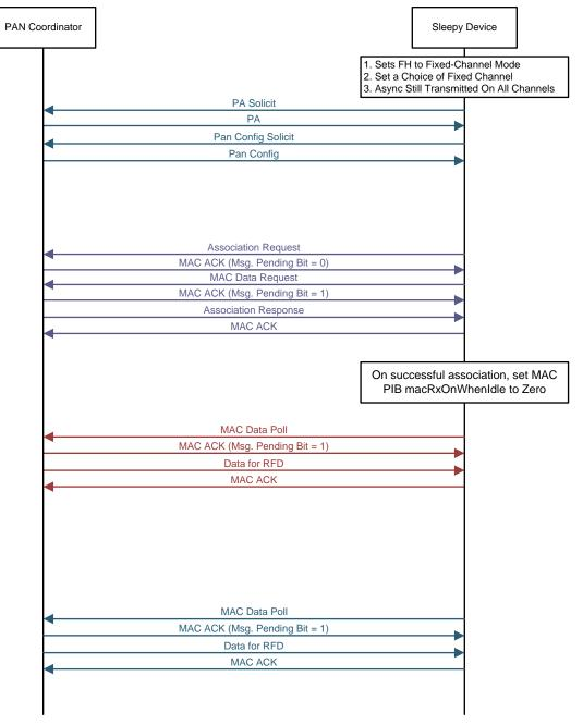
Figure 4-24. Sleep Mode Operation in Frequency-Hopping Mode
