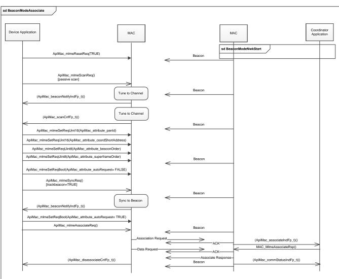
Figure 4-2. Beacon Mode Device Association Sequence
