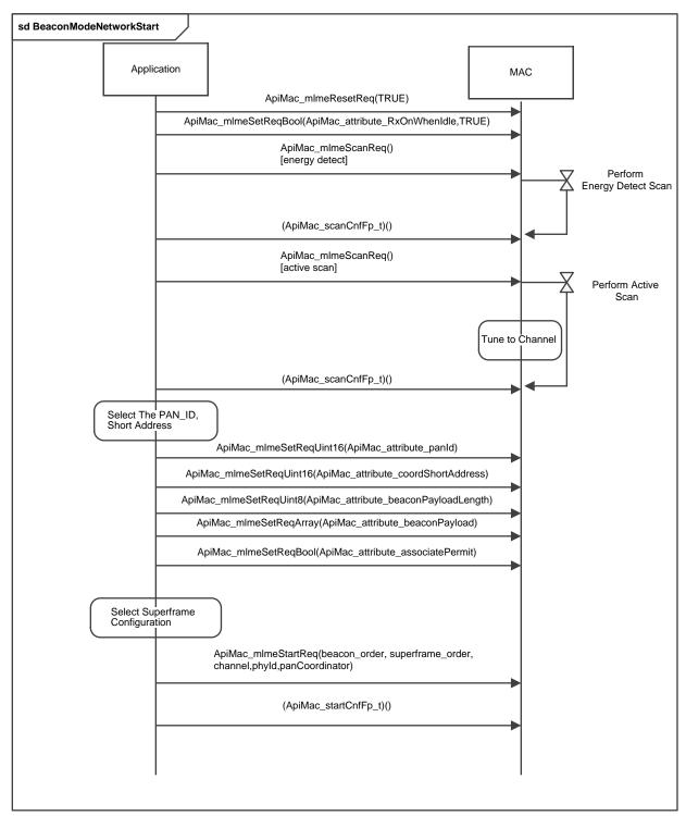
Figure 4-1. Beacon Mode Network Start-Up Sequence
