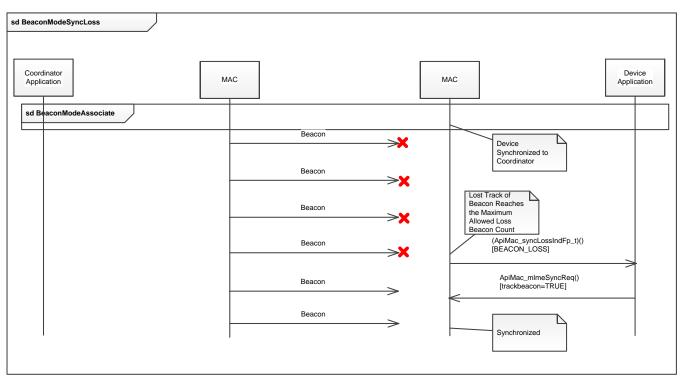
Figure 4-5. Beacon Mode Sync Loss Sequence
