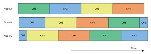
Figure 4-16. Unicast Hopping Sequence
