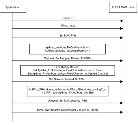
Figure 4-19. Start-Up Sequence of the Device
