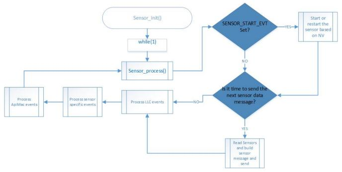
Figure 5-4. Sensor Example Application Task Flow Chart
