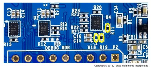
Figure 5-1. CC256XCQFN-EM PCM Role Selection for Audio and Voice Sample Applications
