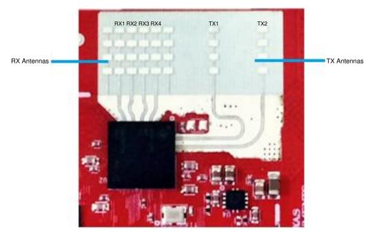
Figure 11. RX and TX Antennas
