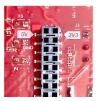
Figure 10. 3V3 and 5V Marking on BoosterPack
