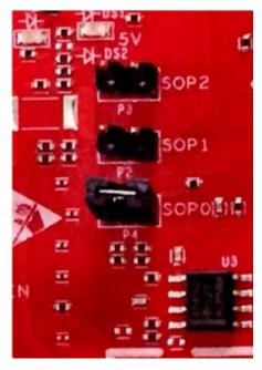
Figure 13. SOP Jumpers
