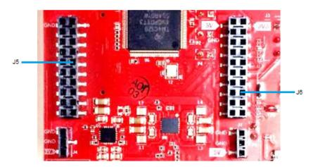
Figure 6. 20-Pin BoosterPack Connectors
