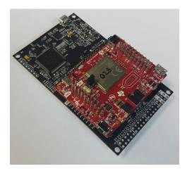
Figure 1-24. BOOSTXL-CC3120MOD Connected to MSP432™ LaunchPad
