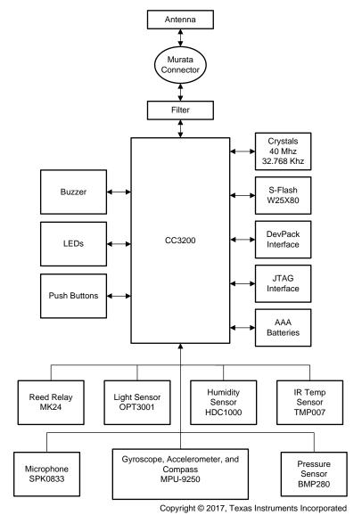
Figure 1. CC3200 SensorTag Block Diagram
