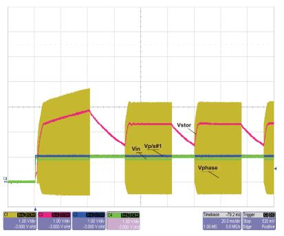
Figure 3. Startup with Battery Less Than UV
