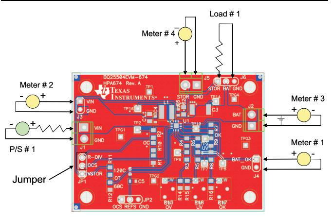
Figure 1. Test Setup for HPA674A (bq25504 EVM)
