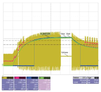
Figure 5. BAT\_OK High/Low 2.8V/2.34V – Ramping Battery from 0V to 3.1V (OV) and Down to 1.8V.
