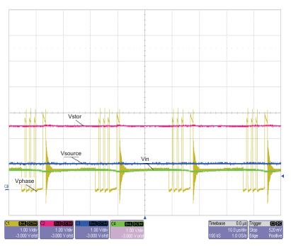
Figure 6. Basic Switching Converter, Vin = 1V, Vbat = 2.5V
