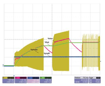
Figure 2. Startup with no Battery and 10k Load
