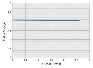
Figure 10. Output Voltage Versus Load Current
