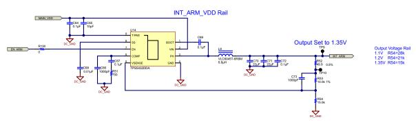
Figure 22. Power Module ARM Supply Circuit
