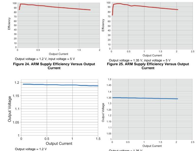
Figure 26. Output Voltage Versus Load Current
