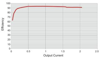
Figure 6. Measured Efficiency Versus Output Current
