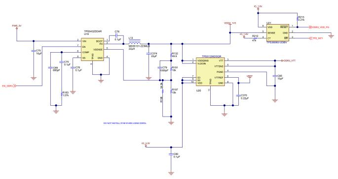
Figure 34. DDR3 Power Supply and Support Circuitry from the Processor Board
