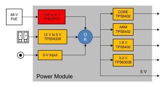
Figure 2. Power Module Block Diagram
