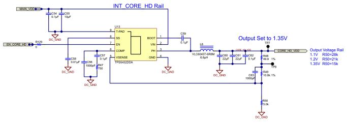
Figure 23. Power Module Core Supply Circuit
