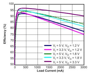
Figure 12. TPS5432 Efficiency Curve
