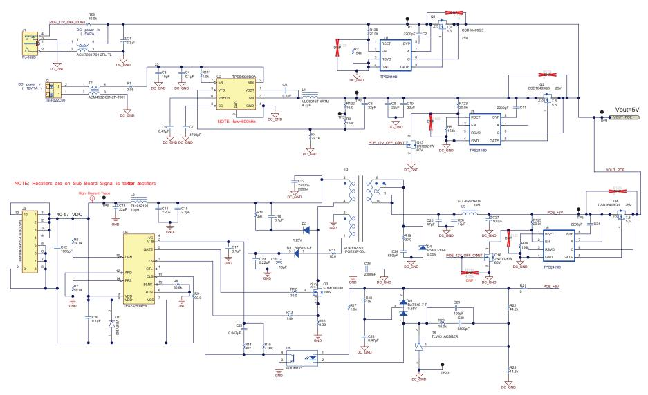
Figure 5. Power Module Input Voltage Circuits
