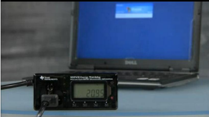
Laptop Active Mode = 20.95 Watts
