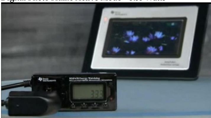
Digital Photo Frame Active Mode = 3.33 Watts
