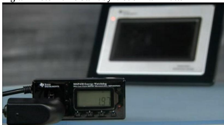
Digital Photo Frame Standby Mode = 1.97 Watts
