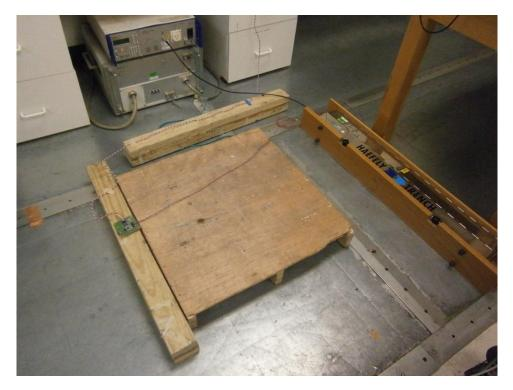
Figure B-4: EFT Test Setup
