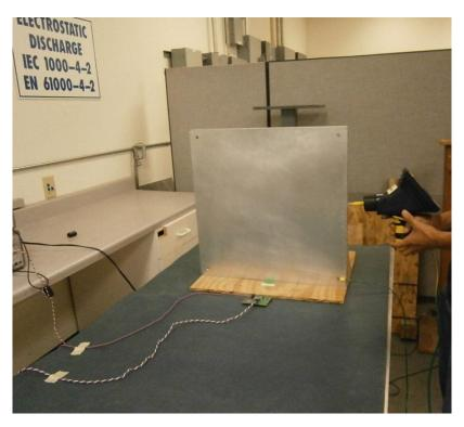
Figure B-2: 8kV ESD Vertical Contact Discharge
