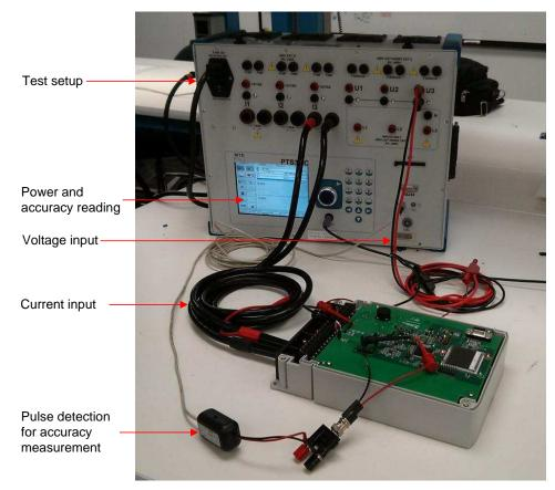
Figure 14. Test Setup Connections
