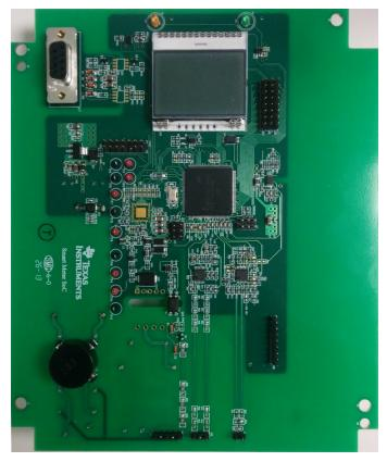
Figure 9. Top View of the Single-Phase Energy Meter EVM
