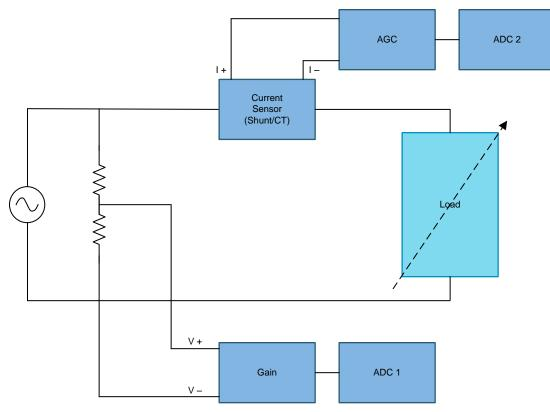
Figure 1. Typical Connections Inside an Electricity Meter
