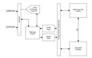
Figure 2. Block Diagram of Concerto-Based Electricity Meter
