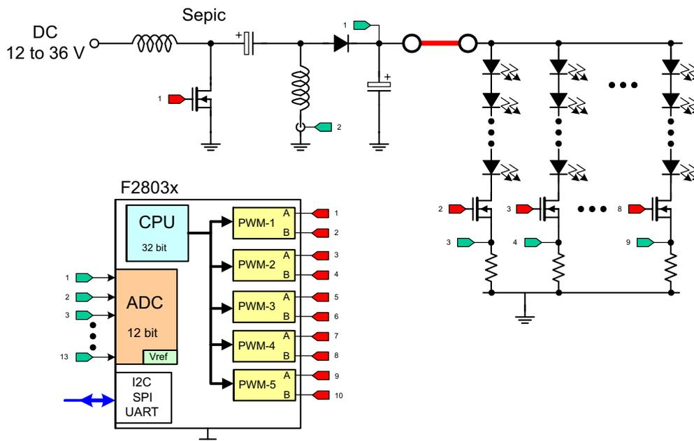
**Figure 4. DC-DC LED Lighting Board Block Diagram with F28035**
