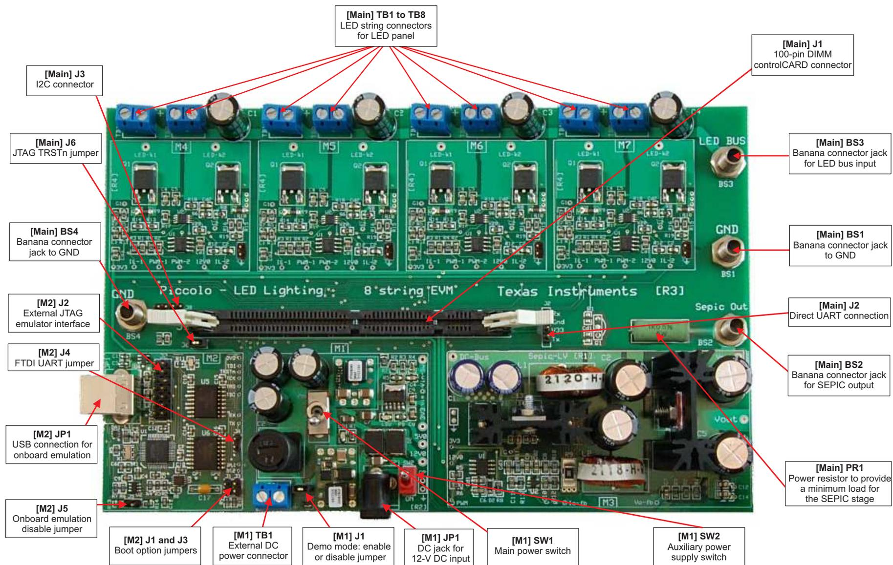
Figure 5. DC-DC LED Lighting Kit Jumpers and Connectors Diagram
