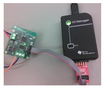
Figure 4. PCB Module With CC Debugger Connected and Ready to Download
