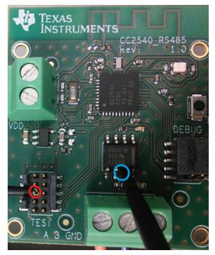
Figure 11. Logic Analyzer Connected to P0\_6 (Red) and Either A or B (Blue)
