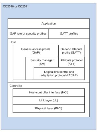
Figure 5. Software Architecture of BLE Device
