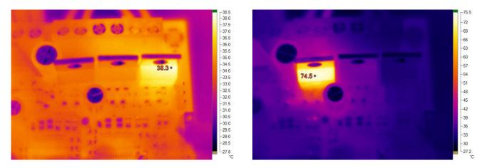
Figure 15. CSD18534KCS Temperatures, Extruder Resistors on the Left and Heated Bed on the Right
