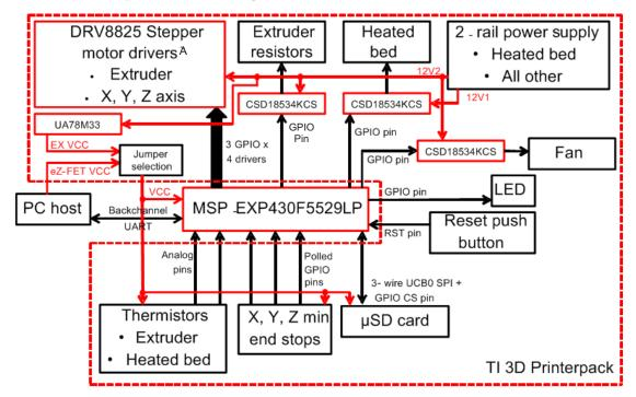
Figure 2. 3D Printerpack Block Diagram
