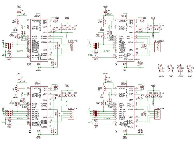
Figure 26. Stepper Drivers Schematic
