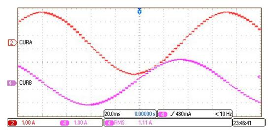
Figure 13. Output Current vs. Step Input for Maximum Driver Operation
