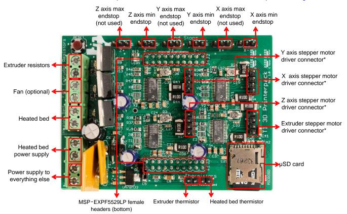
\*Stepper motor connectors can be flipped if motion on 3D printer is opposite of that expected \*\*µSD card functionality has yet to be implemented
