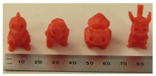
Figure 17. Small Figurines Printed to Demonstrate Small Feature Sizes
