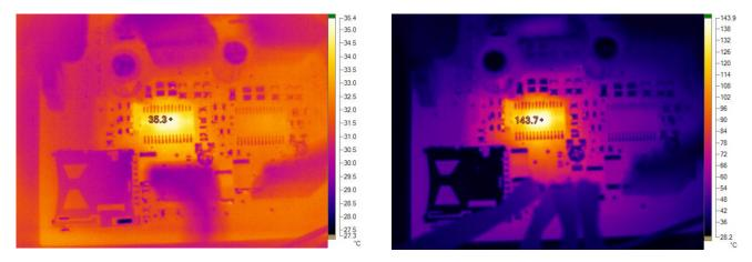
Figure 14. DRV8825 Temperatures, Printer Operation on the Left and Maximum Operation on the Right
