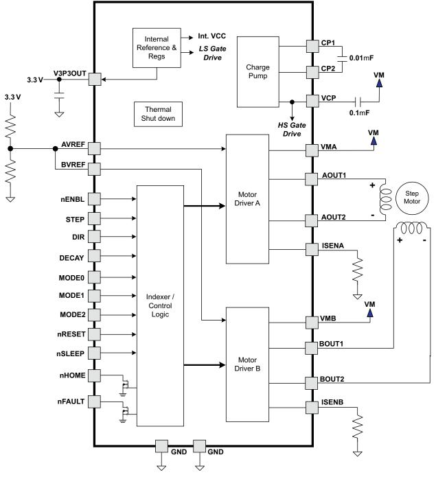
Figure 3. DRV8825 Functional Diagram
