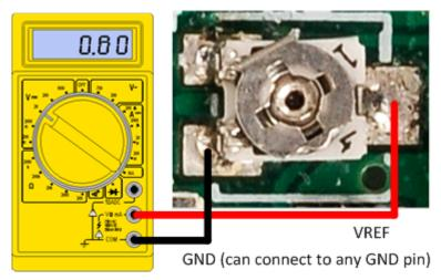
Figure 7. Tuning the VREF Potentiometers
