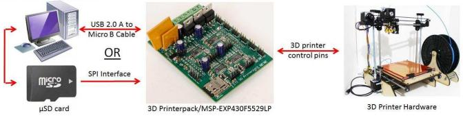
Figure 1. 3D Printer System Diagram
