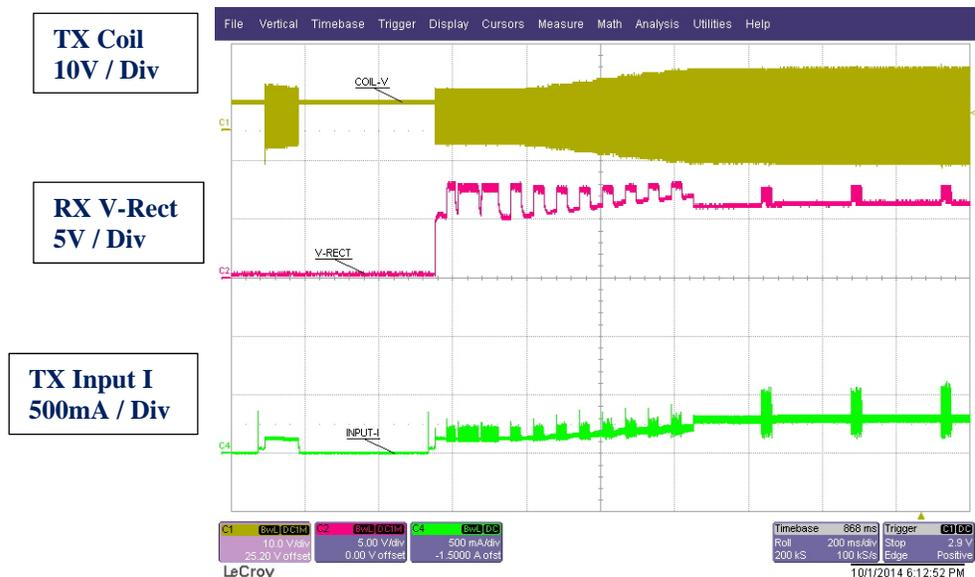
Figure 6 Start Up into 100mA load
