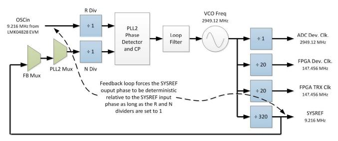
Figure 4. LMK04828 in Single-Loop 0-Delay Mode
