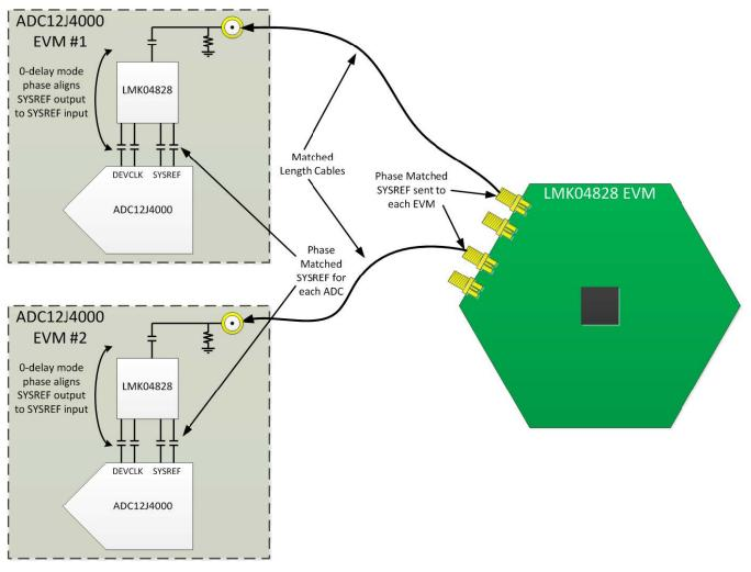
Figure 2. Block Diagram of Clocking Scheme
