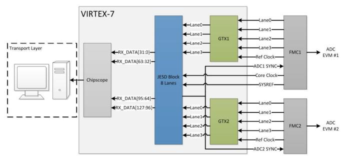
Figure 5. Block Diagram of the VC707 Firmware
