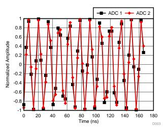
Figure 8. Sampled Signals at 2140 MHz With Complex Mixer Enabled (NCO Frequency = 2070 MHz)
