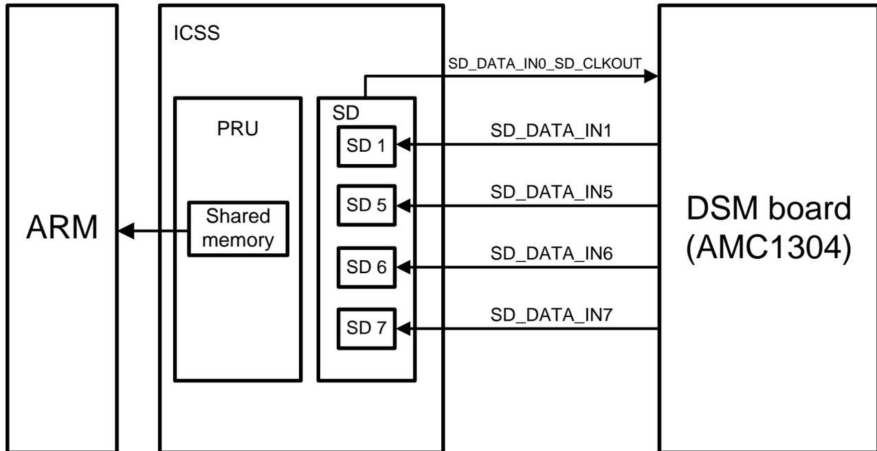
**Figure 18. Application Interface With PRU Sigma-Delta Firmware**
