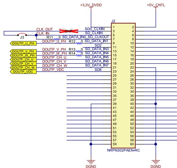
Figure 12. 2x30 Connector Interface With AM437x IDK
