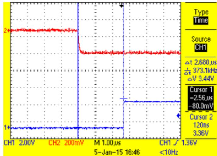
Figure 49. Short Circuit Signal Applied to AMC1304 (Red) and Signal From AM437x (Blue)
