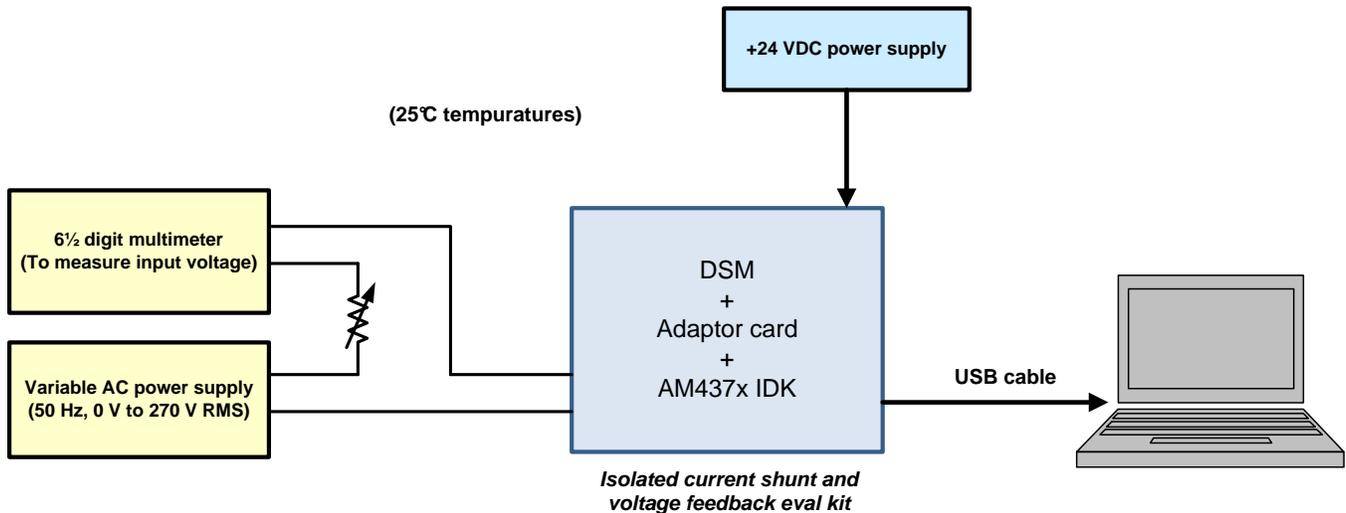
Figure 45. Test Setup for AC Current Measurement Accuracy
