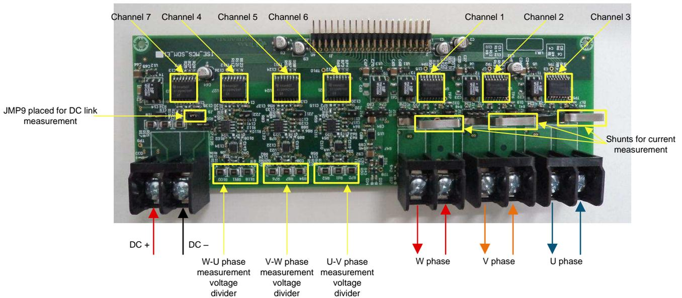
Figure 7. DSM Board
