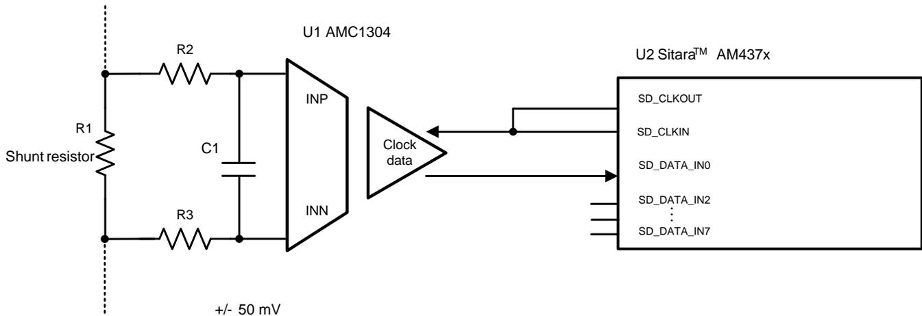
**Figure 3. Current Measurement Using AMC130x and Sitara AM437x Processor**
