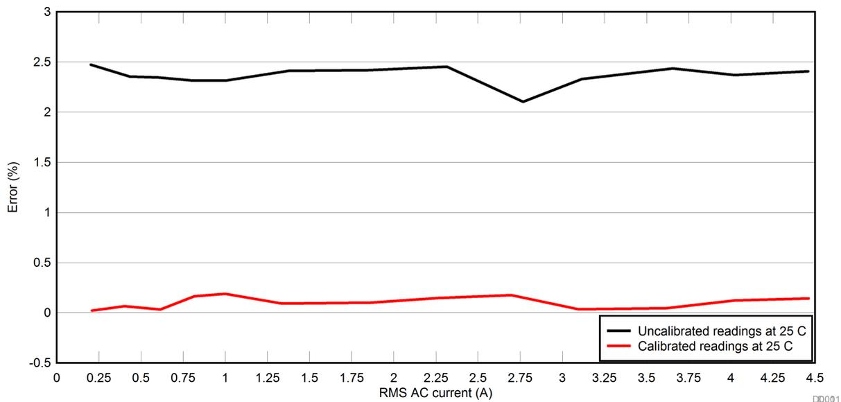
Figure 46. AC Current versus Error
