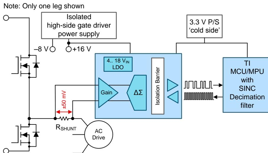
**Figure 2. Delta-Sigma Modulator in Three-Phase Inverters**
