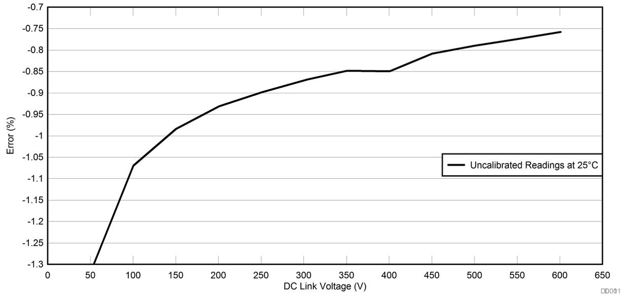
Figure 43. DC Link Voltage versus Error, Uncalibrated Readings at 25°C
