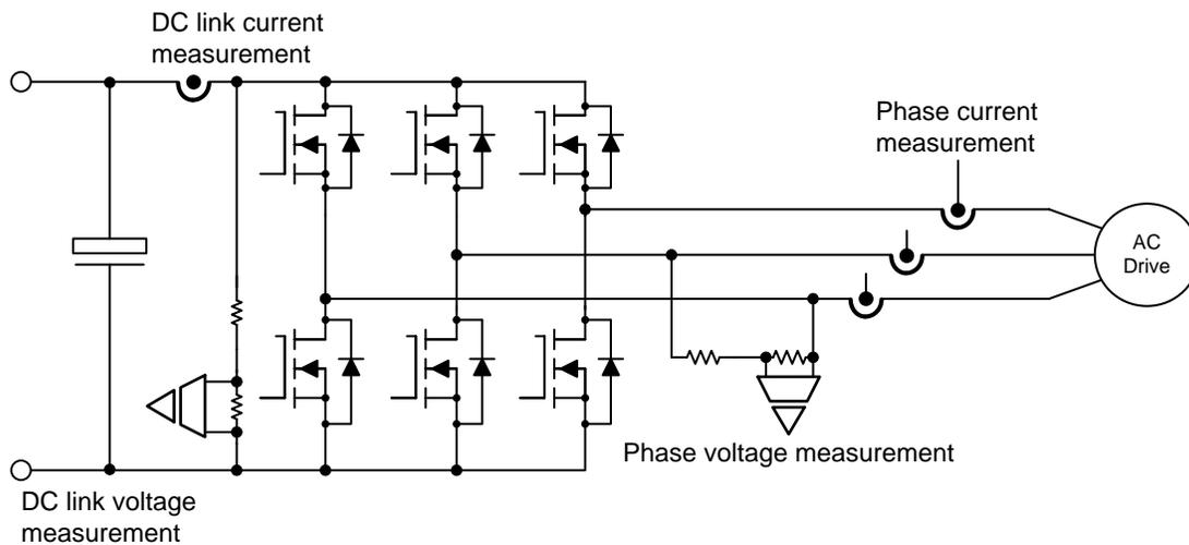
**Figure 1. Current and Voltage Measurements in Three-Phase Inverters**
