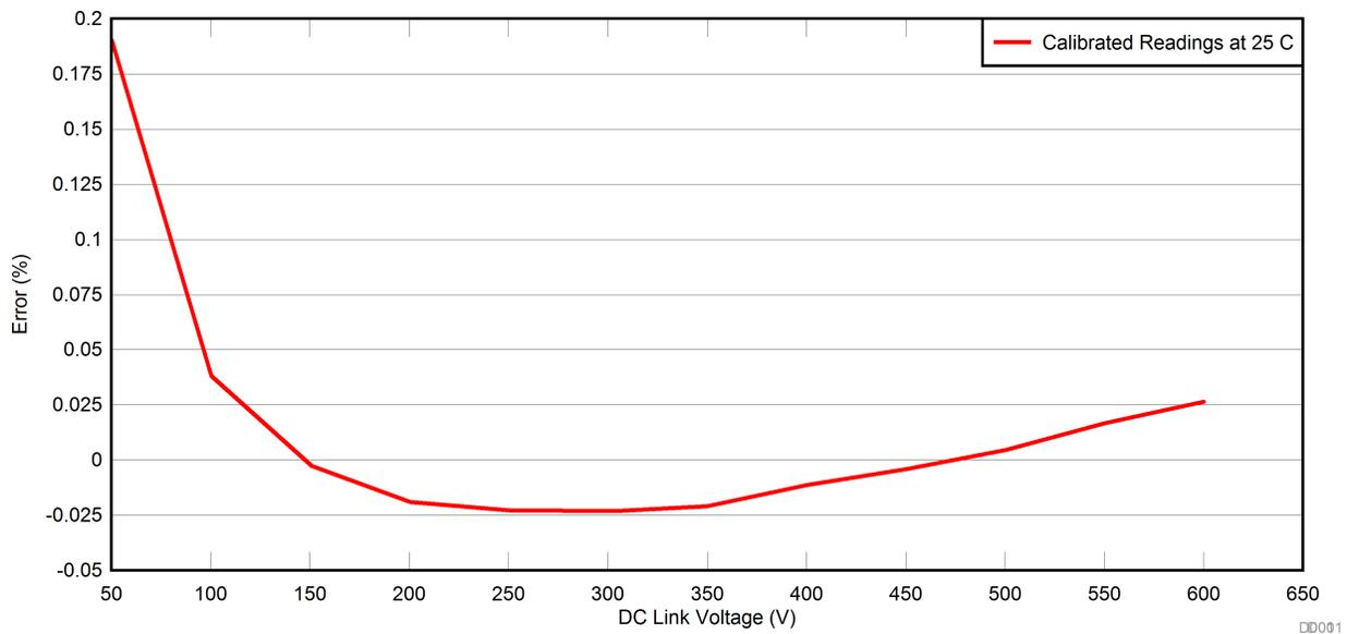
Figure 44. DC Link Voltage versus Error
