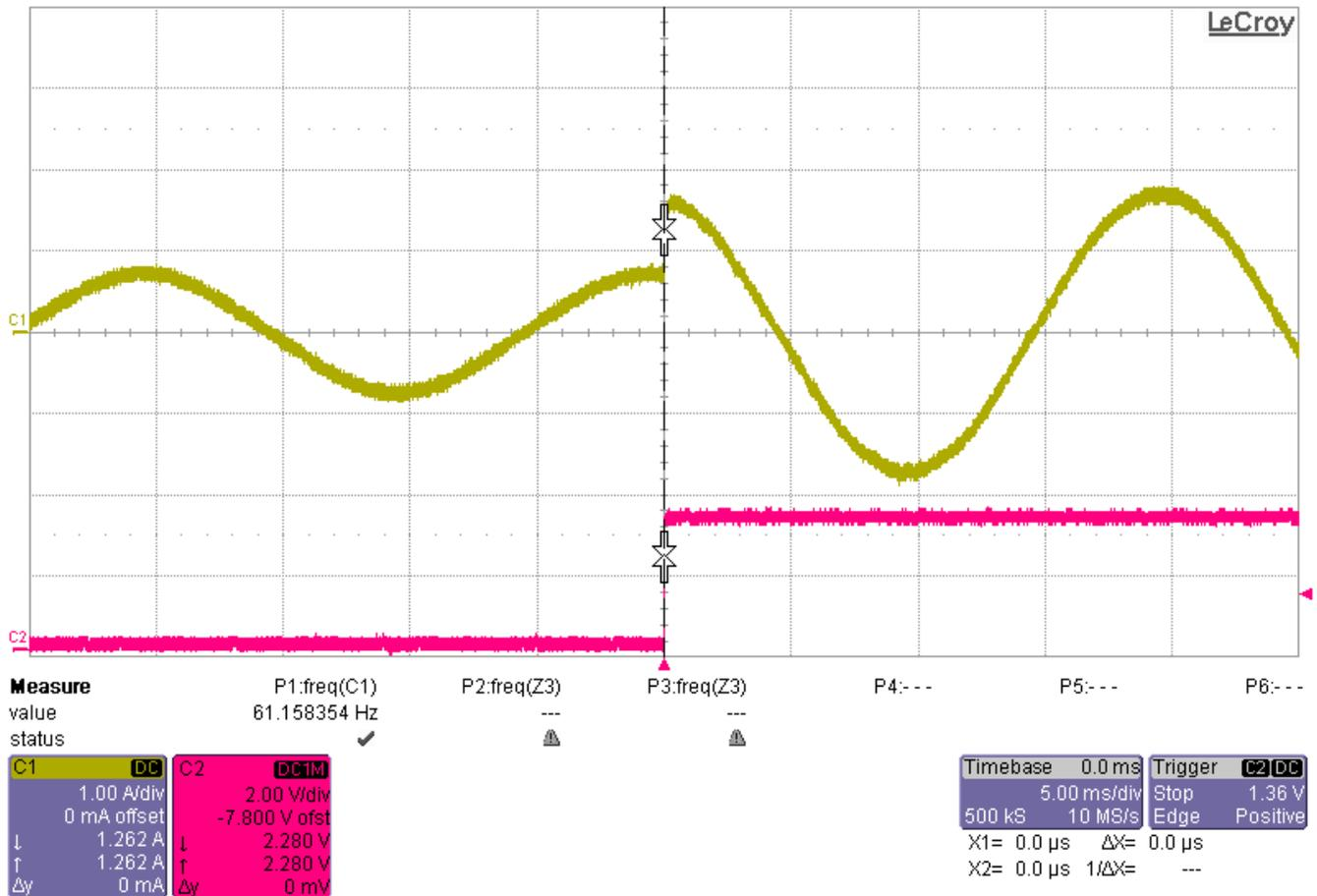
Figure 48. Short Circuit Current Waveform (Yellow) and Signal From AM437x (Red)
