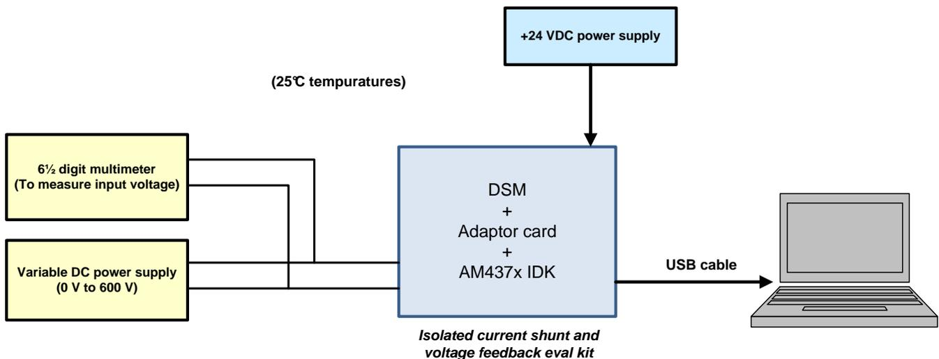
Figure 42. Test Setup for DC Link Voltage Measurement Accuracy
