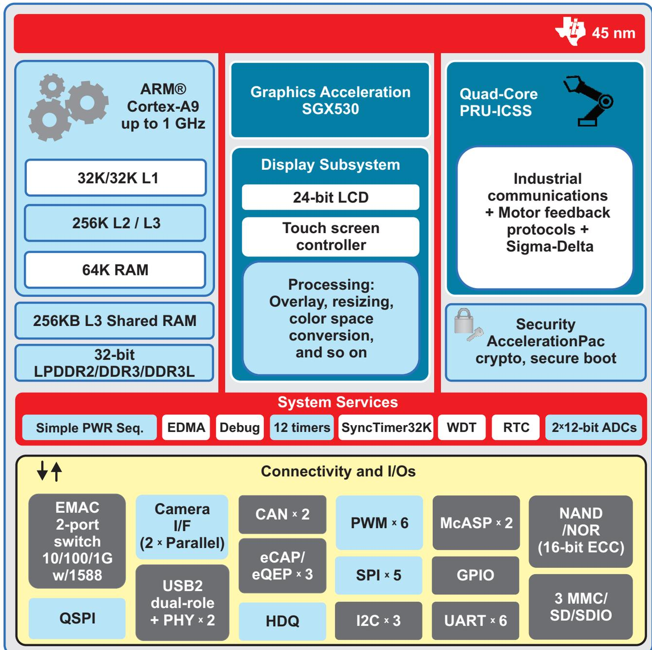
**Figure 13. AM437x Functional Block Diagram**
