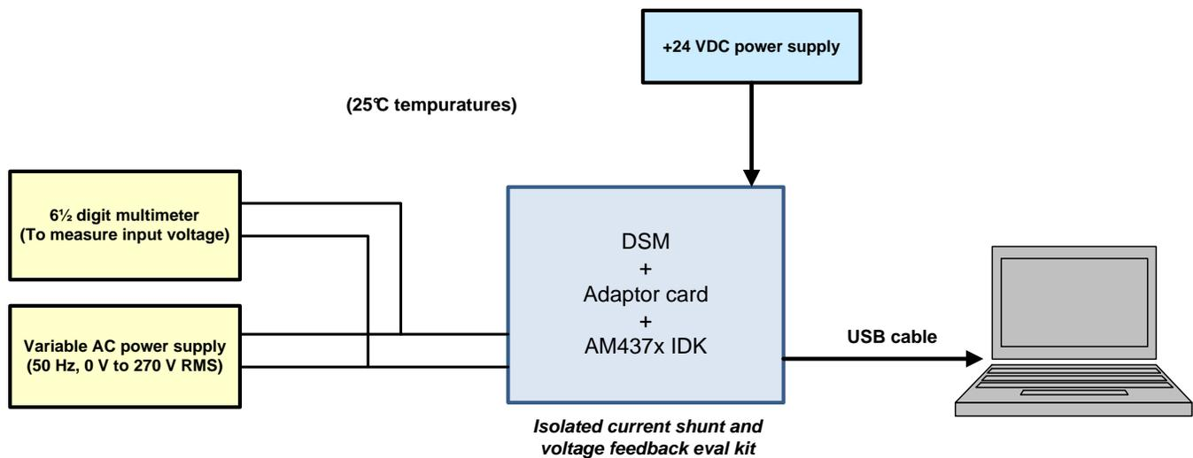
Figure 40. Test Setup for AC Voltage Measurement Accuracy
