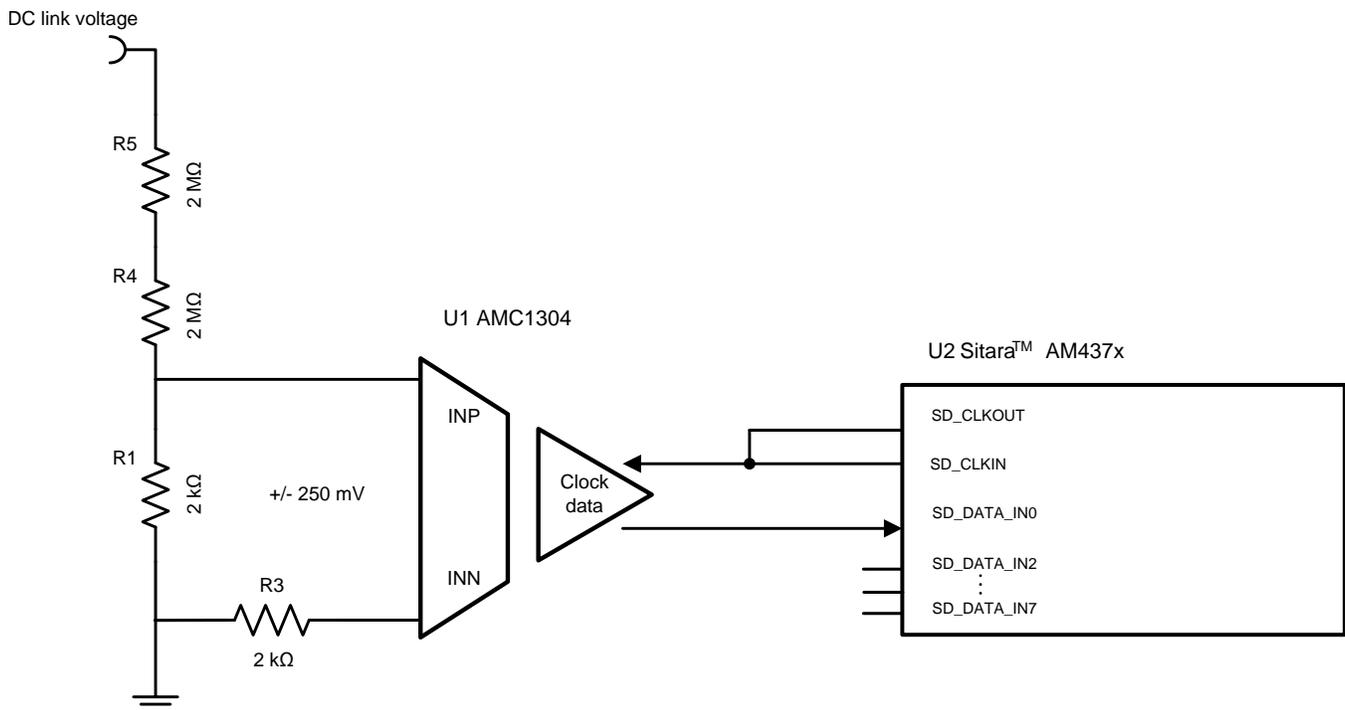
**Figure 4. Voltage Measurement Using AMC130x and Sitara AM437x Processor**
