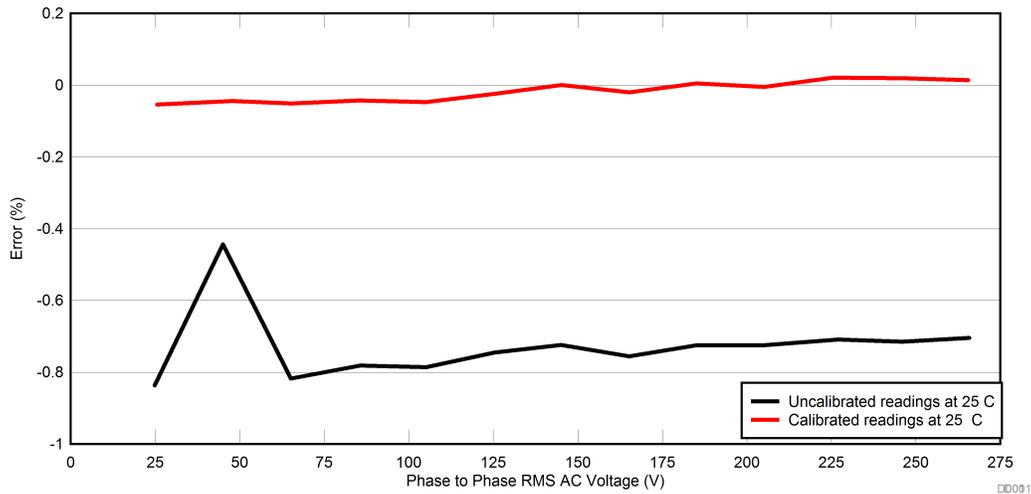
Figure 41. Phase-to-Phase Voltage versus Error
