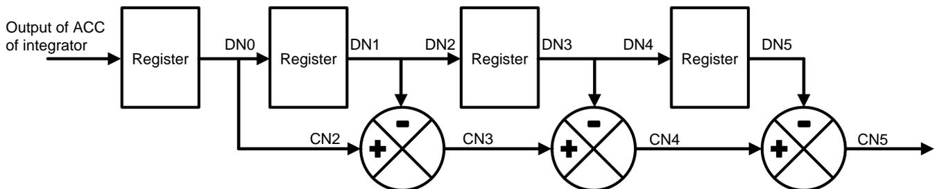
**Figure 17. Sinc3 Filter Differentiation Implementation in PRU**
