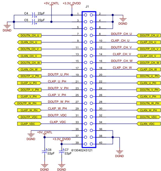
Figure 11. 2x10 Connector Interface With DSM Board
