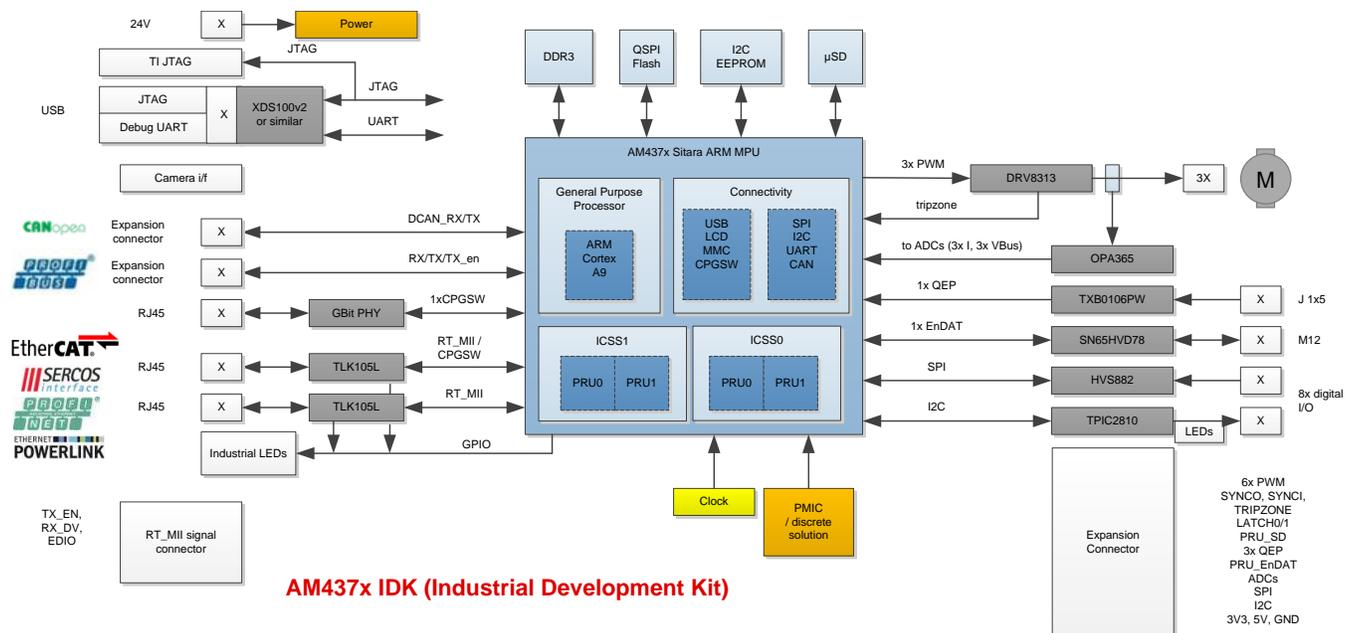
**Figure 8. Block Diagram of AM437x IDK**
