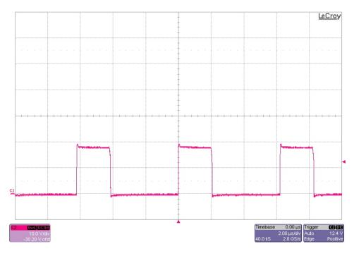
The photo below shows the FET switching voltage (TP2) for an input voltage of 16V and a 1.05A load. The converter is operating in DCM. (10V/DIV, 2uS/DIV)
