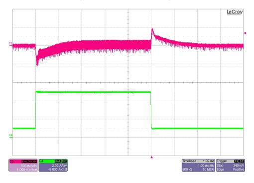
The photo below shows the 12V output voltage (ac coupled) when the load current is stepped between 3A and 5A. Vin = 12V. (200mV/DIV, 2A/DIV, 1mS/DIV)
