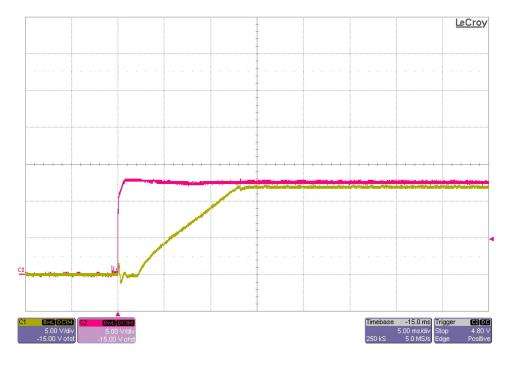
The photo below shows the output voltage startup waveform after the application of 12V in. The 12V output was loaded to 5A. (5V/DIV, 5mS/DIV)
