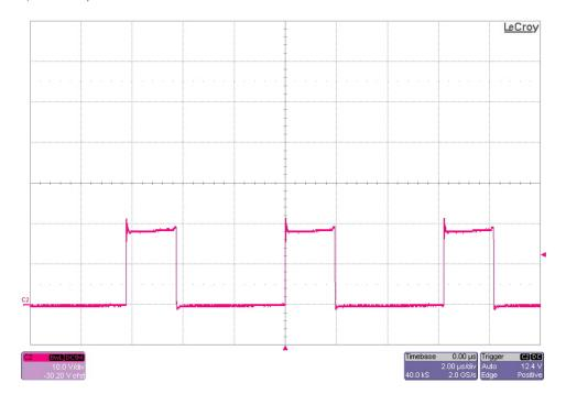
The photo below shows the FET switching voltage (TP2) for an input voltage of 16V and a 5A load. (10V/DIV, 2uS/DIV)
