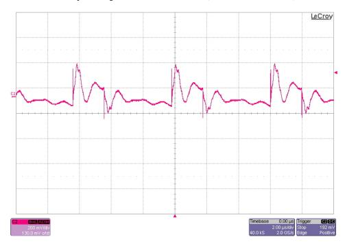
The 12V output ripple voltage (AC coupled) is shown in the figure below. The image was taken with the output loaded to 5A. The input voltage is set to 16V. (200mV/DIV, 2uS/DIV)
