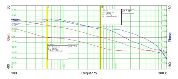
The plot below shows the loop gain with the input voltage set to 6V and 16V and the output set to 1A.
