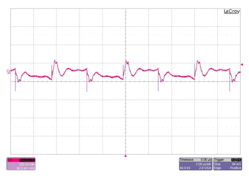
The 12V output ripple voltage (AC coupled) is shown in the figure below. The image was taken with the output loaded to 1A. The input voltage is set to 12V. (50 mV/DIV, 2 uS/DIV)
