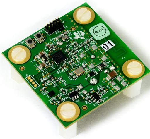
**Figure 7. Humidity and Temperature Sensor Node for Star Networks Enabling 10+ Year Coin Cell Battery Life Reference Design Hardware (Top View)**
