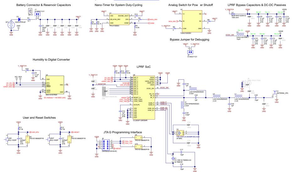
Figure 21. Humidity and Temperature Sensor Node for Star Networks Enabling 10+ Year Coin Cell Battery Life Schematic
