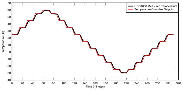
Figure 20. HDC1000 Measured Temperature Data and Environmental Chamber Set Point
