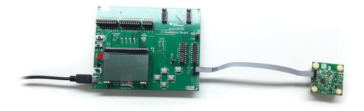
Figure 10. Connection of SmartRF06 Evaluation Board and TI Designs Hardware for Programming/Debugging
