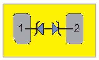
Figure 6. TPD1E10B06 Device Configuration
