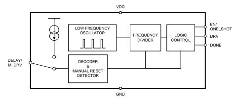
Figure 4. TPL5110 Functional Block Diagram
