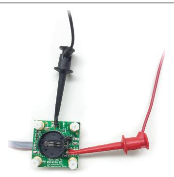
Figure 9. Configuration of Jumpers and Power for Programming and Debugging
