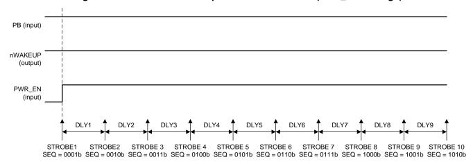
Figure 3. TPS65218D0 Power-Up from SUSPEND State (PWR\_EN Set High)
