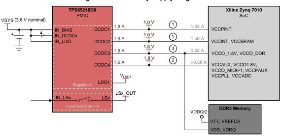
Figure 2. 3.6-V Battery Supply Diagram
