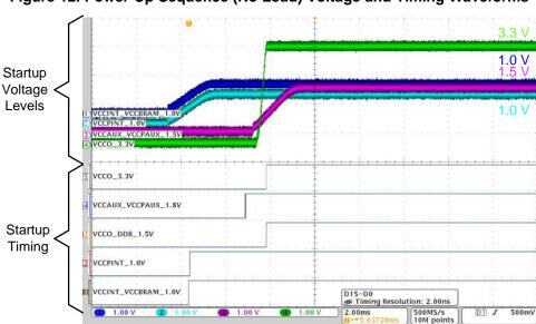
Figure 12. Power-Up Sequence (No Load) Voltage and Timing Waveforms
