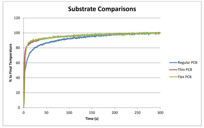
Figure 9: Overall Substrate Comparison
