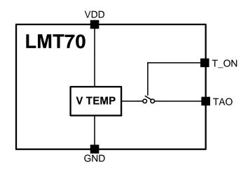
Figure 1: LMT70 Block Diagram
