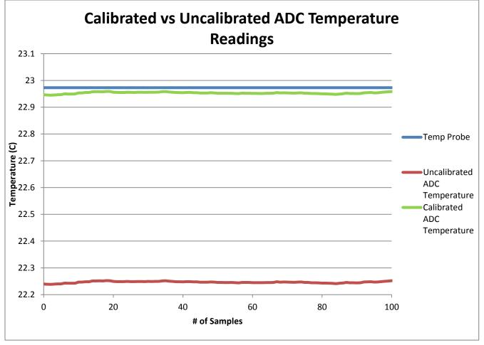
Figure 3: Temperature Measurements with ADC Calibration
