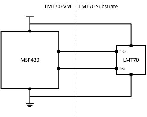
Figure 5: Block Diagram
