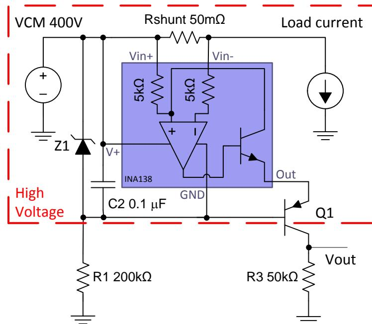
**Figure 3 - Schematic**
