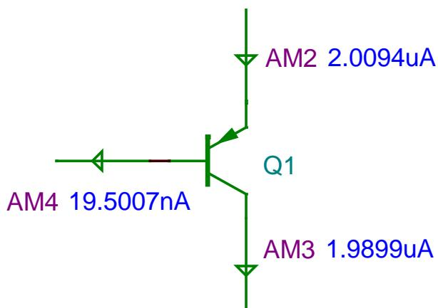
Figure 4 – Current through the PNP Transistor
