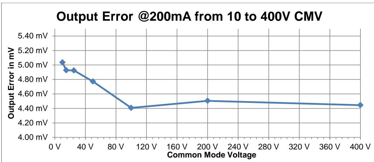
**Figure 1: Output Error over Common Mode Voltage**
