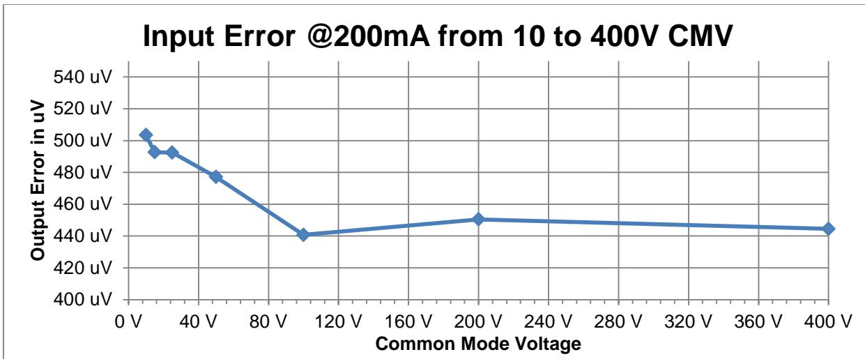
**Figure 2: Input Error over Common Mode Voltage**
