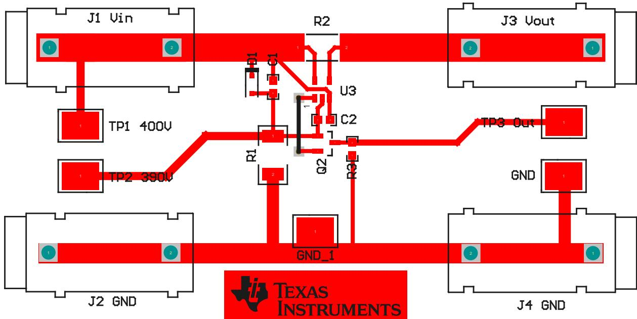
**Figure 6 - PCB Layout**
