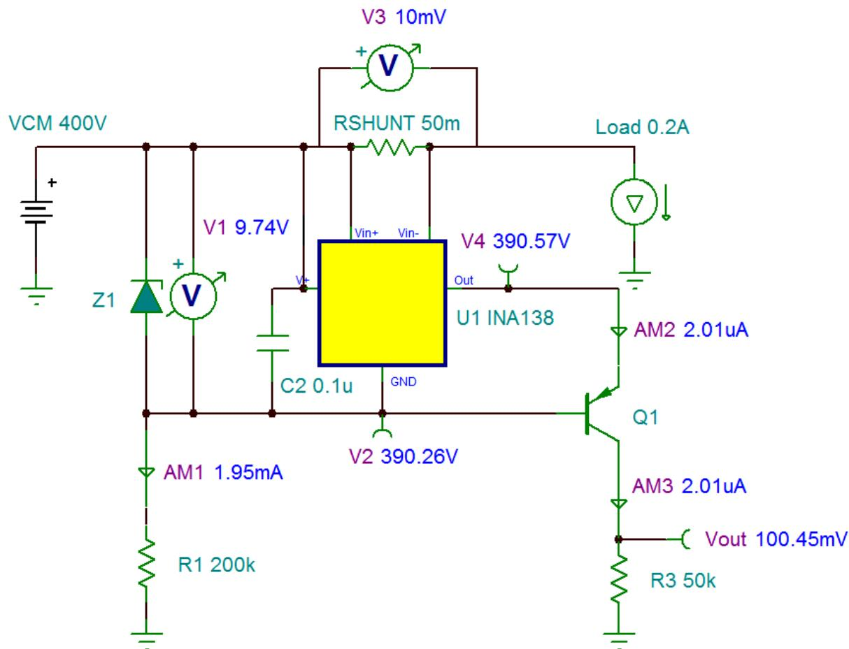
**Figure 5 - DC Circuit Simulation**
