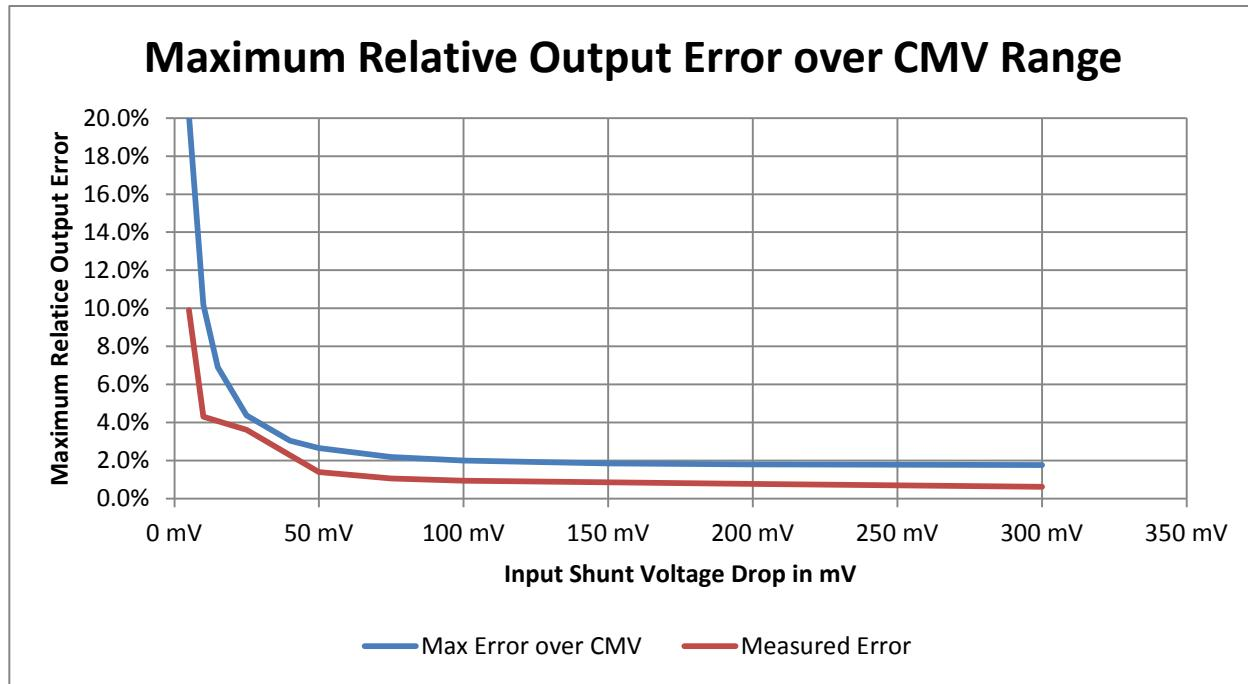
**Figure 7 – Maximum Relative Output Error**
