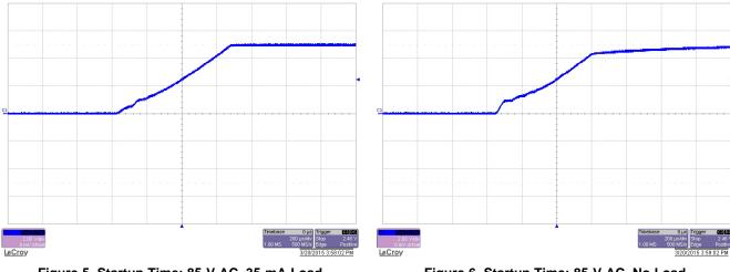
Figure 5. Startup Time: 85-V AC, 35-mA Load
