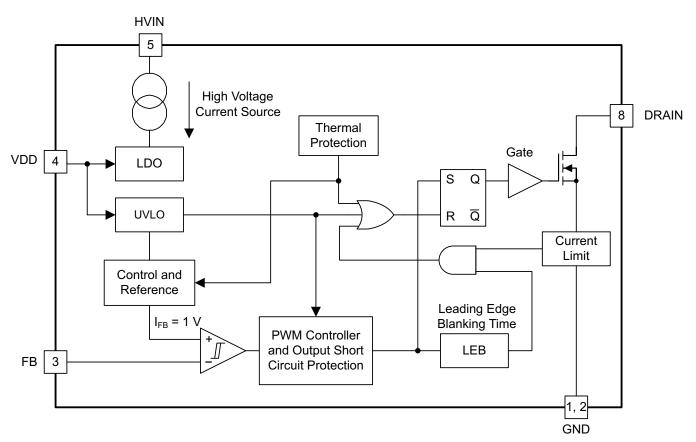
Figure 2. UCC28880 Functional Block Diagram
