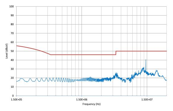
Figure 18. EMI Results: 120-V AC/60-Hz Line, 5-V DC/40 mA
