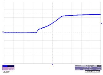
Figure 8. Startup Time: 120-V AC, No Load
