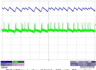
Ch3: LDO input voltage (2.0 V/div, 500 μs/div, DC coupling) Ch4: LDO output voltage (10 mV/div, 500 μs/div, AC coupling)
