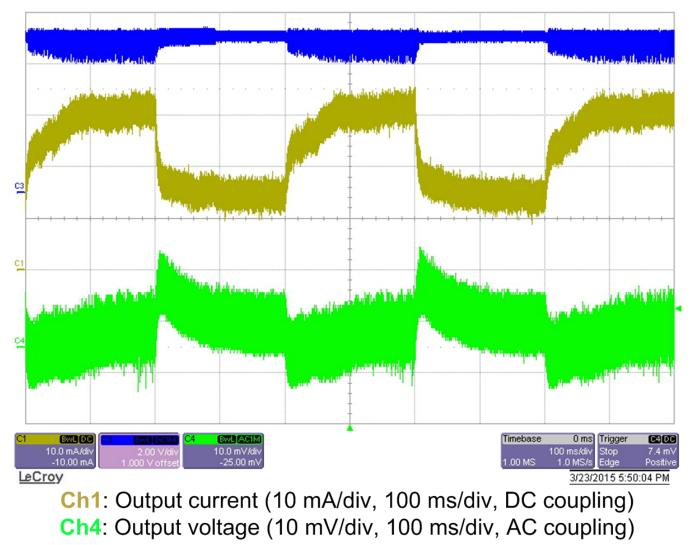
Figure 16. Output Voltage Transient Response
