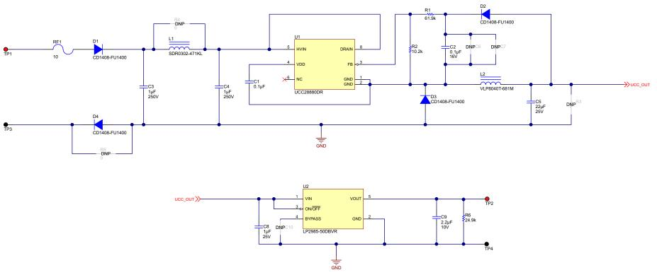
Figure 20. AC-to-DC Power Supply Schematics
