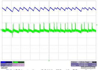
**Ch3**: LDO input voltage (2.0 V/div, 500 μs/div, DC coupling) **Ch4**: LDO output voltage (10 mV/div, 500 μs/div, AC coupling)
