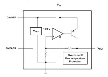
Figure 3. LP2985 Functional Block Diagram
