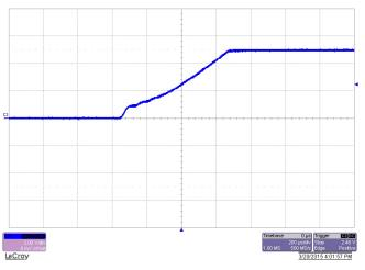
Figure 7. Startup Time: 120-V AC, 35-mA Load
