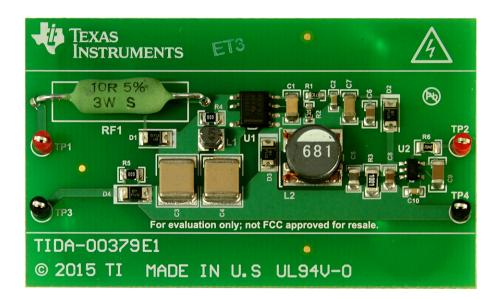
Figure 4. 110-V AC to 5-V DC @ 30-mA Non-Isolated Power Supply Reference Design Hardware
