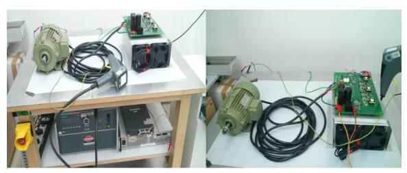
Figure 113. EUT/AUX Equipment on Insulated Sheet
