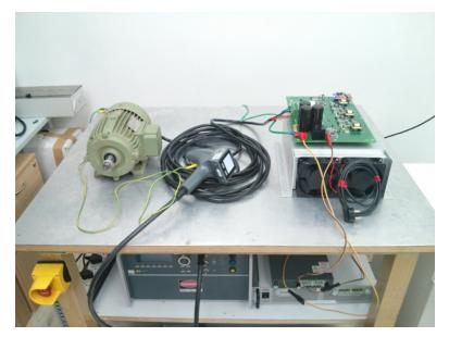
Figure 116. Test Configuration 2: EUT/AUX Equipment on Reference Plane
