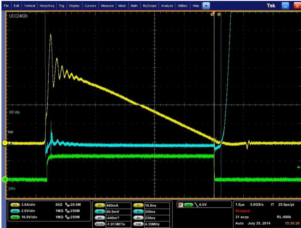
Figure 9. SR VDS, Isec, and SR Gate Drive at 115V, Full Load
