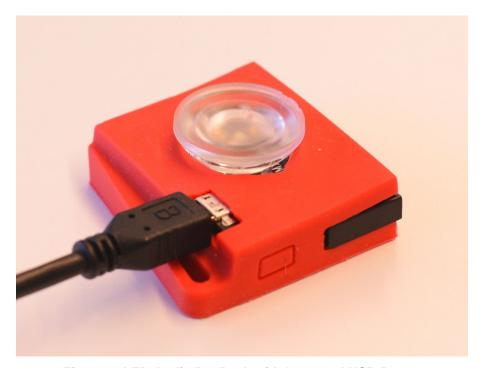
Figure 7. LED Audio DevPack with Lens and USB Power
