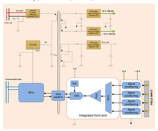
Figure 1. Generic Illustration of Analog Input Module
