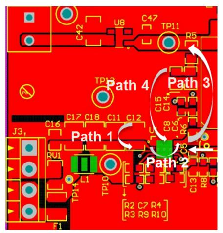
Figure 19. Isolating Converter Primary Side
