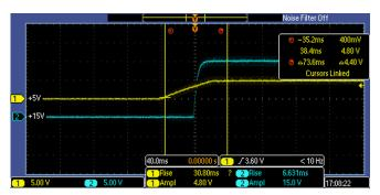
Figure 7. Startup of  $V_{J5} = 15 \text{ V}$  at  $V_{IN} = 24 \text{ V}$
