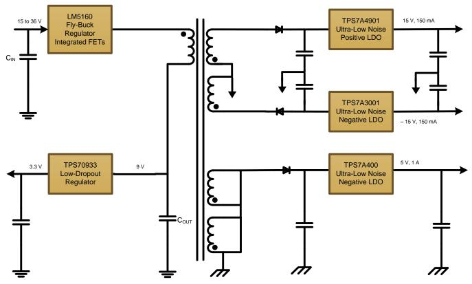
Figure 2. TIDA-00401 Isolated Power Supply Diagram for Analog Input Module
