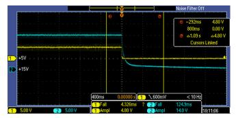
Figure 10. Shutdown at  $V_{IN} = 24 \text{ V}$
