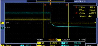
Figure 9. Shutdown of at V<sub>IN</sub> = 15 V
