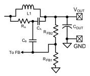
Figure 5. Typical Noise Amplification Scheme
