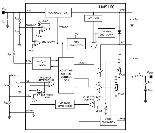
Figure 3. LM5160 Circuit Diagram
