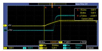
Figure 8. Startup of  $V_{J5}$  = 15 V at  $V_{IN}$  = 36 V
