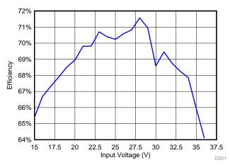
Figure 14. Overall Efficiency versus Input Voltage
