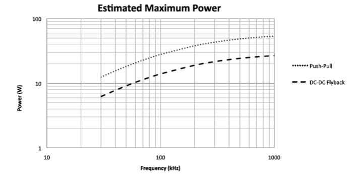
Figure 4. EFD15 Power versus Frequency Curve (Würth 070-5939)
