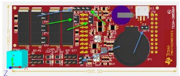
J1 will disconnect the output of the 5V regulator from the header pins. These pins can also be used to measure current out of the 5V regulator by adding a current shunt or meter in series
