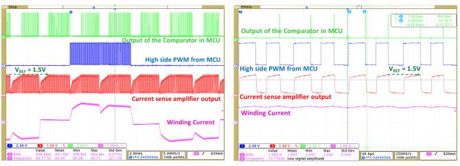
Figure 45. Cycle-By-Cycle Current Limit Using Hardware Features of MSP430F5132
