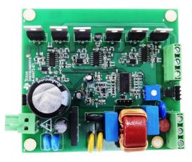
016 230-V/250-W, Hi-η Sensorless Brushless DC Motor Drive With 30% Reduced Bulk Capacitor Reference Design Copyright © 2015–2016, Texas Instruments Incorporated
