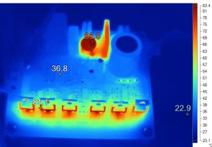
Figure 34. Thermal Image of Board at 250-W Inverter Power and 300-V DC Input
