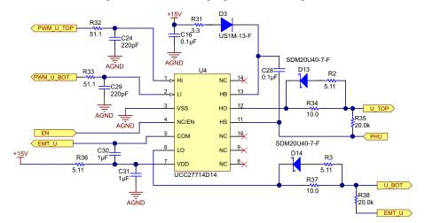
Figure 5. Gate Driver Circuit Using UCC27714
