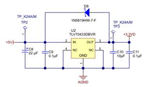
Figure 13. 3.3-V Power Supply Using LDO TLV70433
