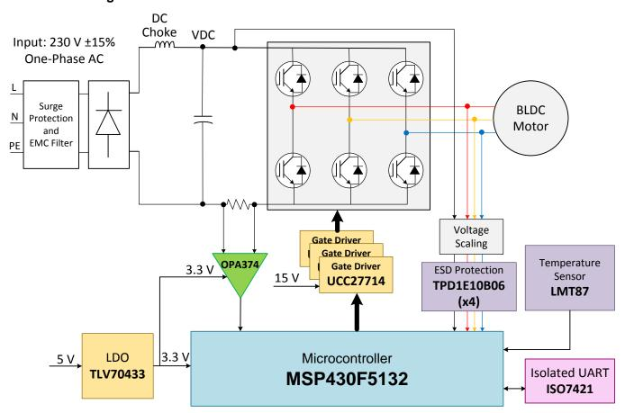
Figure 1. Block Diagram of Mains-Powered 250-W BLDC Drive (TIDA-00472)
