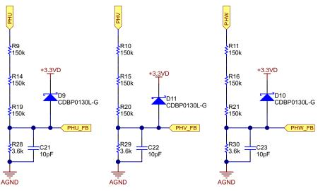
Figure 6. Motor-Winding Voltage Sensing
