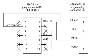
Figure 19. Programming Interface Between the Programmer Kit and MSP430F5132
