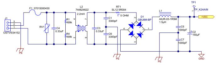
Figure 2. AC-DC Converter Schematic
