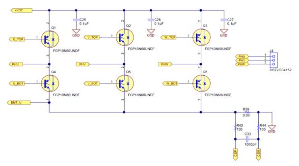
Figure 3. Three-Phase Inverter of Power Stage
