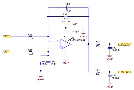
Figure 9. Current Sense Amplifier Using OPA374
