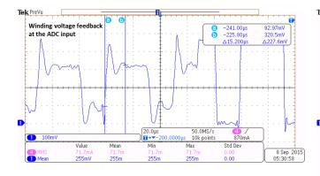
Figure 51. Oscillations in Winding Voltage Feedback for a High inductance Motor
