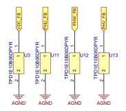
Figure 8. ESD Protection on Voltage Sensing Lines
