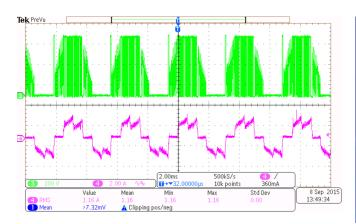
Figure 33. Winding Voltage and Winding Current of Motor at 250-W Inverter Power
