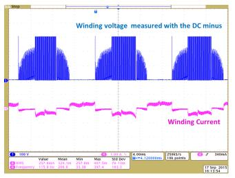
Figure 49. Winding Voltage and Winding Current of Motor at 1000 RPM
