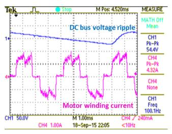
Figure 36. DC-Bus Voltage Ripple and Winding Current of Motor at 250-W Inverter Power (Zoomed-In to One Cycle of Voltage Ripple)
