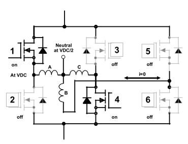
Figure 22. Motor Neutral voltage During PWM On-Period
