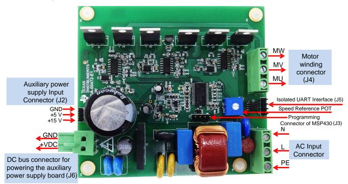
Figure 17. TIDA-00472 PCB Connectors
