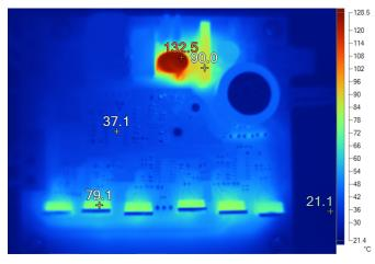
Figure 37. Thermal Image of Board at 250-W Inverter Power
