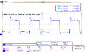
Figure 52. Oscillations in Winding Voltage Feedback for a Low inductance Motor
