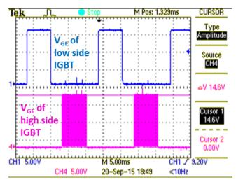
Figure 30. High-Side and Low-Side PWM Output From UCC27714
