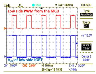
Figure 31. V<sub>GE</sub> of Low Side IGBT and PWM From MCU
