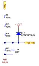
Figure 7. DC-Bus Voltage Sensing
