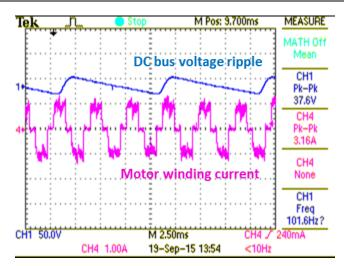
Figure 38. DC-Bus Voltage Ripple and Winding Current of the Motor at 150 W Inverter Power
