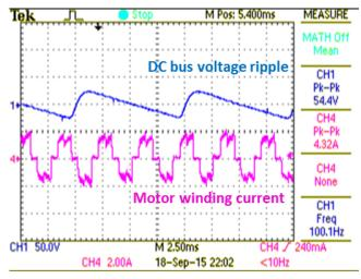
Figure 35. DC-Bus Voltage Ripple and Winding Current of Motor at 250-W Inverter Power
