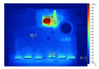
Figure 39. Thermal Image of Board at 150-W Inverter Power
