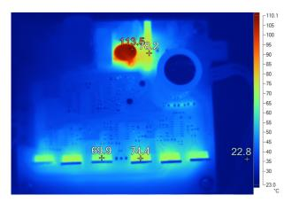
Figure 40. Thermal Image of Board at 200-W Inverter Power
