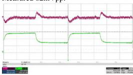
150mA to 420mA load step Slew Rate = 50mA/usec 50mV/div, 200mA/div, 100usec/div Measured 77mVpp:
