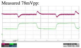
150mA to 420mA load step Slew Rate = 50mA/usec 50mV/div, 200mA/div, 100usec/div
