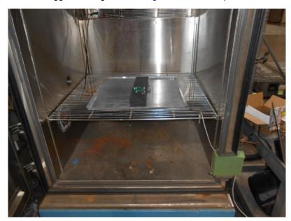
Figure 19. Wireless PIR Motion Detector Temperature and Humidity Test Setup
