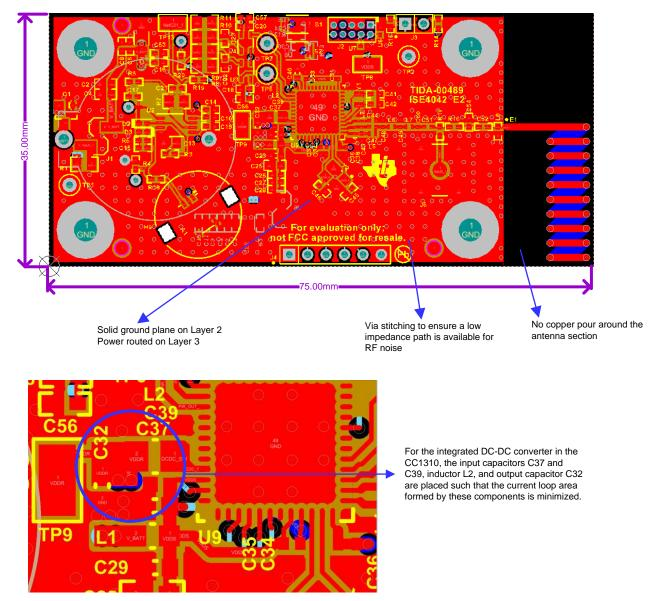
Figure 35. Low-Power PIR Motion Detector Reference Design Layout Guidelines
