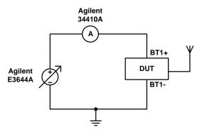
Figure 17. Test Circuit Used for Measuring Supply Current
