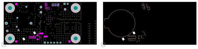
Figure 32. Bottom Solder Mask
