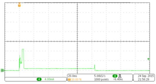
Figure 23. Radio Transmission Event Supply Current (Full Picture)
