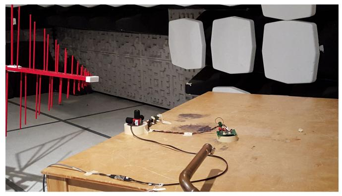
Figure 21. RF Immunity Test Setup
