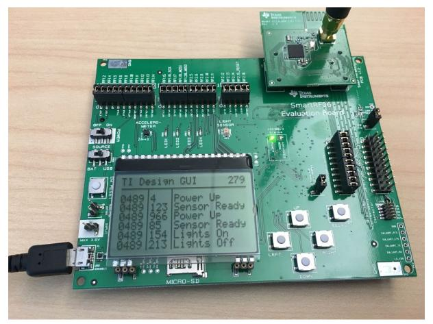
Figure 12. Building Automation Sub-1GHz Sniffer GUI
