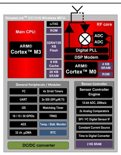
Figure 3. CC1310 Functional Block Diagram
