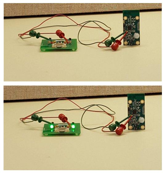
Figure 20. Motion Sensitivity Test Setup (Top: No Motion; Bottom: Motion Detected)
