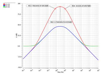
Figure 6. Amplified Filter Simulation Results (Ideal)
