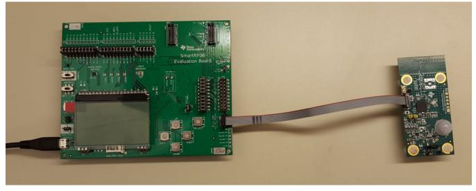
Figure 11. Connection of SmartRF06 Evaluation Board and TI Designs Hardware for Programming and Debugging
