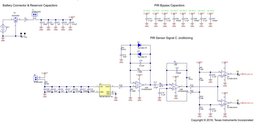
Figure 24. Power and PIR Sensor Schematic
