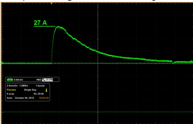
Figure 3. Maxon RE 30 310007 Startup Current
