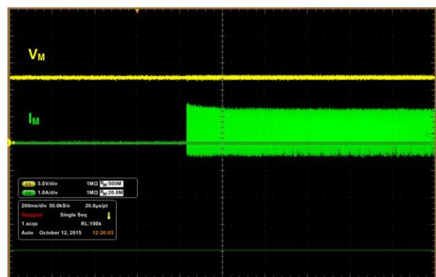
**Figure 2.**  $V_M$  Stable with Current Limiting
