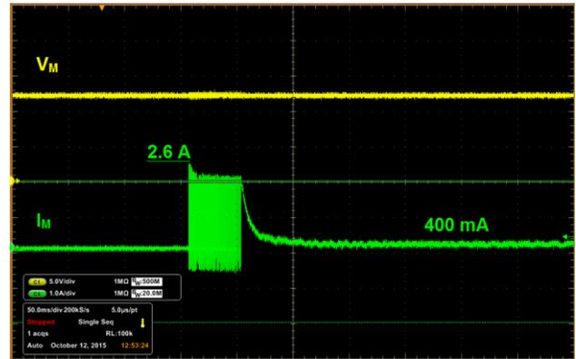
**Figure 6.** Startup and Steady State Current
