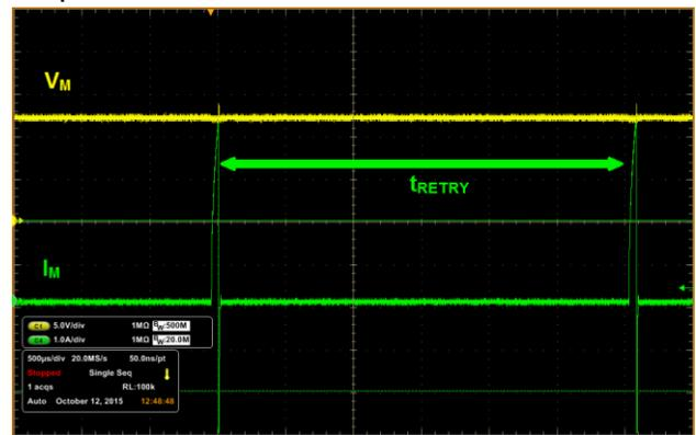
Figure 4. OCL  $t_{RETRY}$  interval
