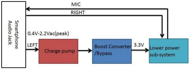
Figure 2: Application Block Diagram
