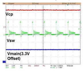
Figure 12: Rload=3.3K Ohm, Boost Converter Switching
