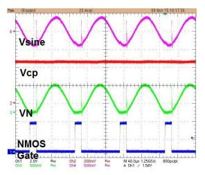
Figure 11: Rload=3.3K Ohm, Charge Pump Switching
