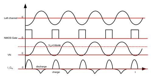
Figure 4: Typical Waveforms of the Charge Pump
