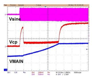
Figure 9: No Load Startup with VMAIN Pre-biased by MIC Voltage
