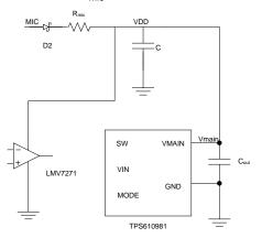
Figure 7: Auxiliary Circuit
