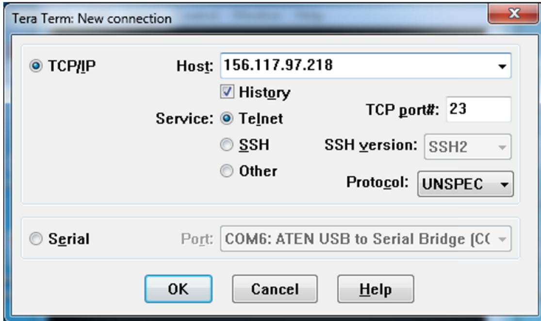
Figure 3. Tera Term: New Connection Setup—TCP/IP
