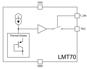
Figure 1. Block Diagram of LMT70A
