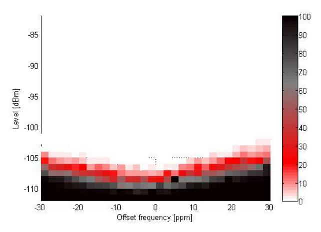
Figure 14. C2-Mode Meter RX Packet Error Rate versus Signal Level versus Frequency Offset (Minimal Deviation of 18.75 kHz)
