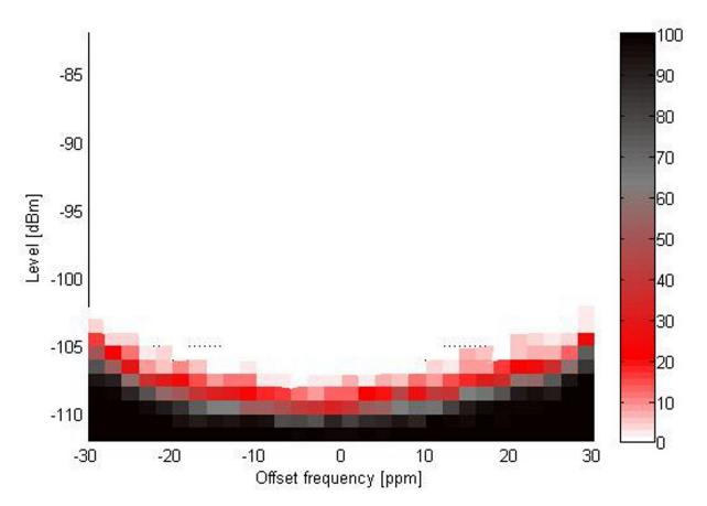
Figure 13. C2-Mode Meter RX Packet Error Rate versus Signal Level versus Frequency Offset (Nominal)
