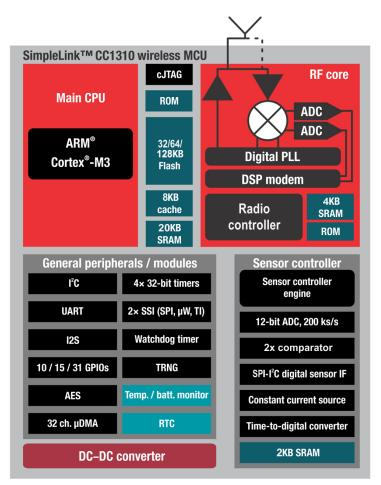
Figure 2. CC1310 Functional Block Diagram
