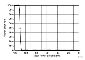
Figure 16. S2-Mode Meter RX Packet Error Rate versus Signal Level
