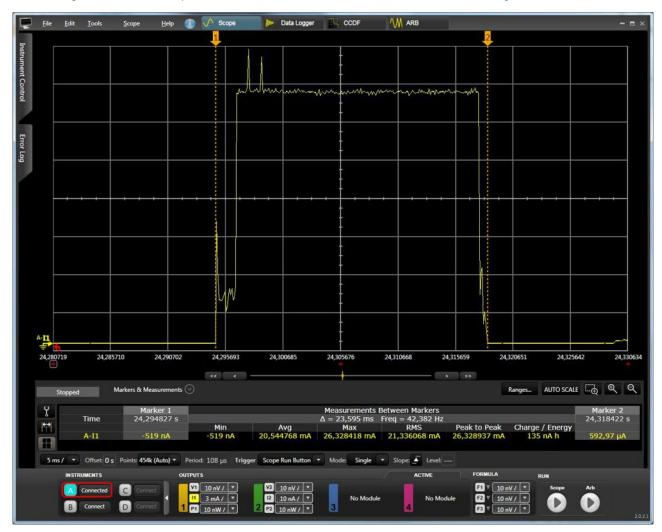
Figure 19. 20.54-mA Average Current During RF Transmission Pulse at 12.5 dBm; MSP430FR4133 is in LPM3; LCD BTL002 is Off
