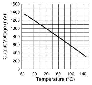
Figure 4. LMT70 Output Transfer Function
