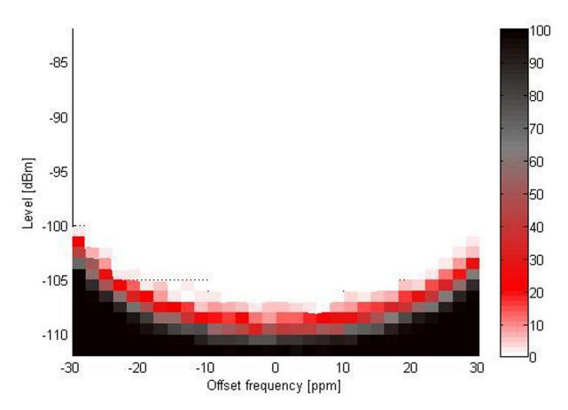
Figure 15. C2-Mode Meter RX Packet Error Rate versus Signal Level versus Frequency Offset (Maximum Deviation of 31.25 kHz)
