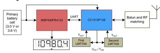
Figure 3. Block Diagram of the TIDA-00838
