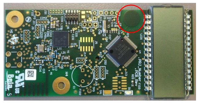
Figure 11. PCB Area for Capacitive Touch (Used to Implement LCD On/Off Functionality)
