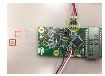
Figure 6. "Small" PCB Layout for LMT70
