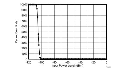
Figure 12. C2-Mode Meter RX Sensitivity for Packet Error Rate (20-Byte Payload) With Nominal Deviation
