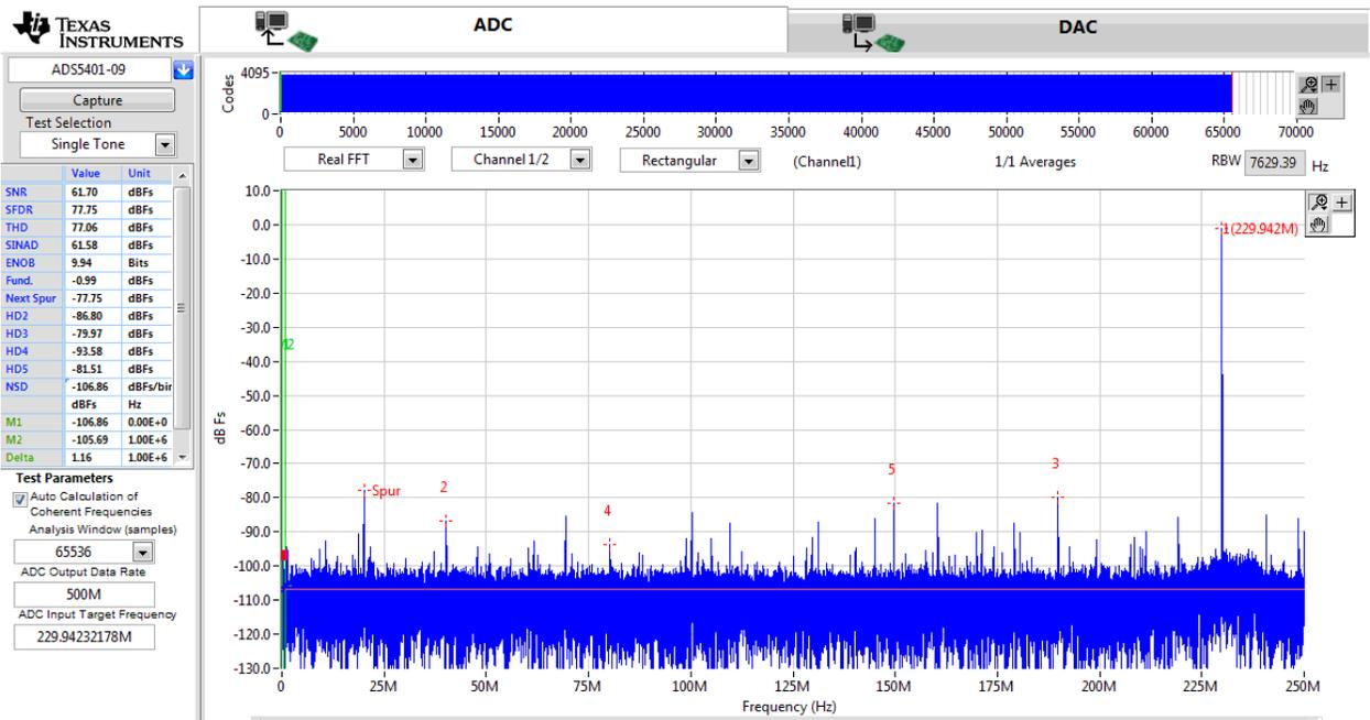
**Figure A-6. ADS5407 powered with SMPSs and 230-MHz signal frequency**
