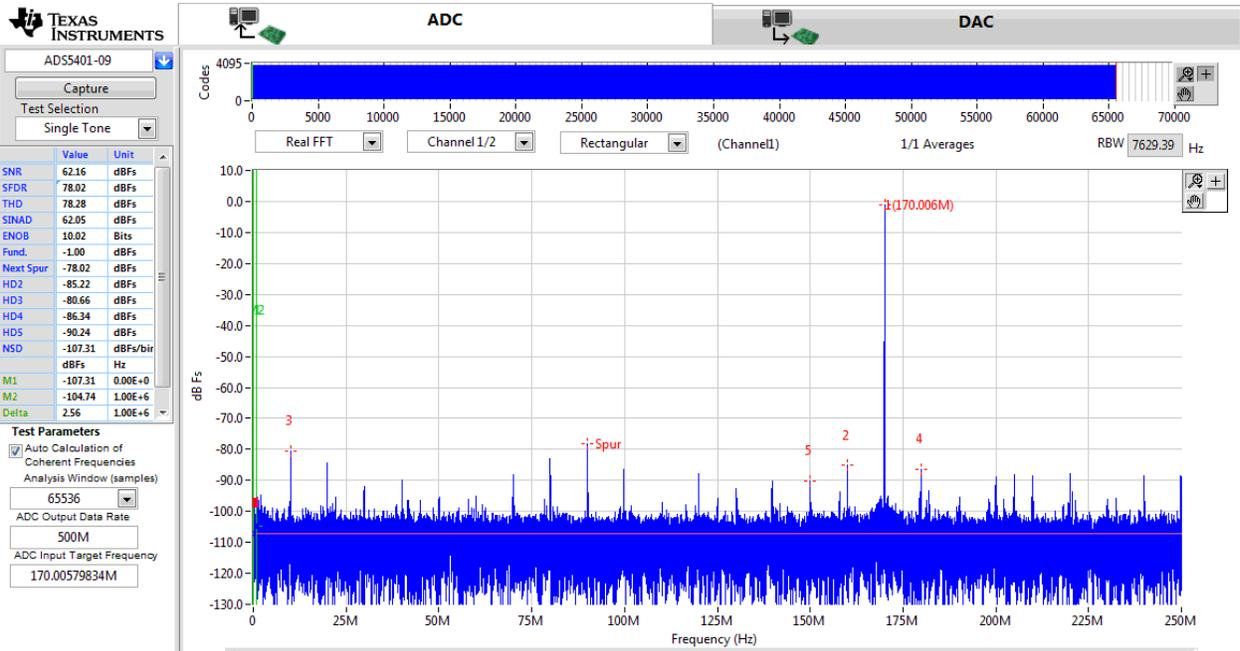
Figure A-3. ADS5407 powered with LDOs and 170-MHz signal frequency
