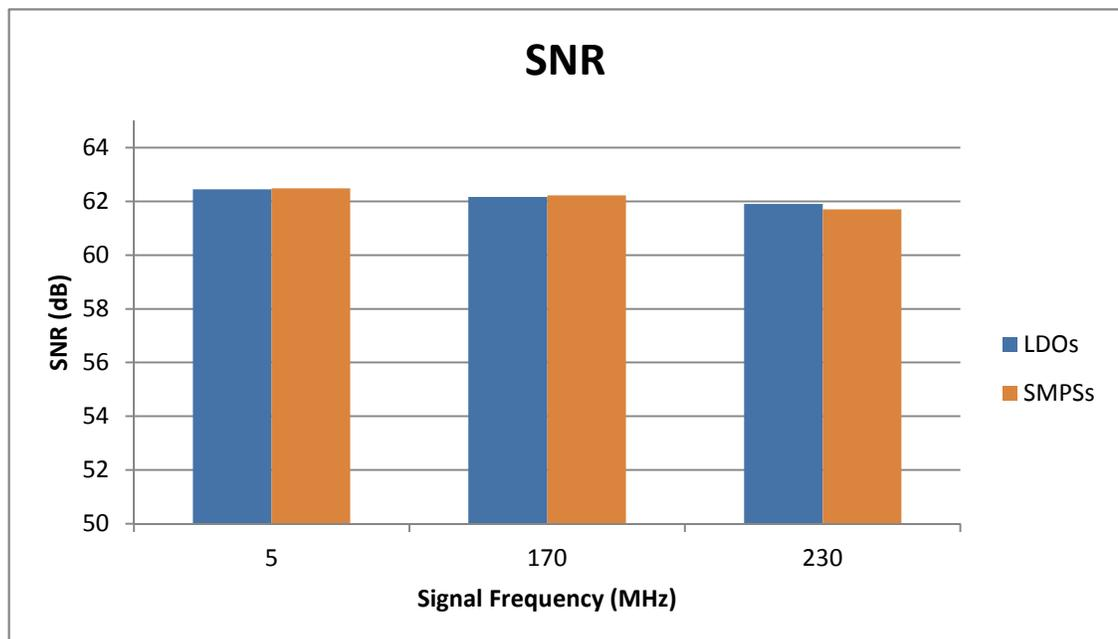
Figure 2. SNR comparison of the LDO power solution to the SMPS power solution
