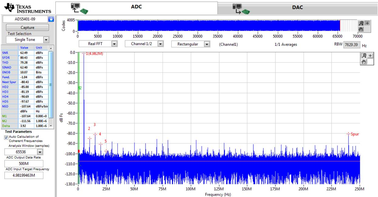
**Figure A-2. ADS5407 powered with SMPs and 5-MHz signal frequency**
