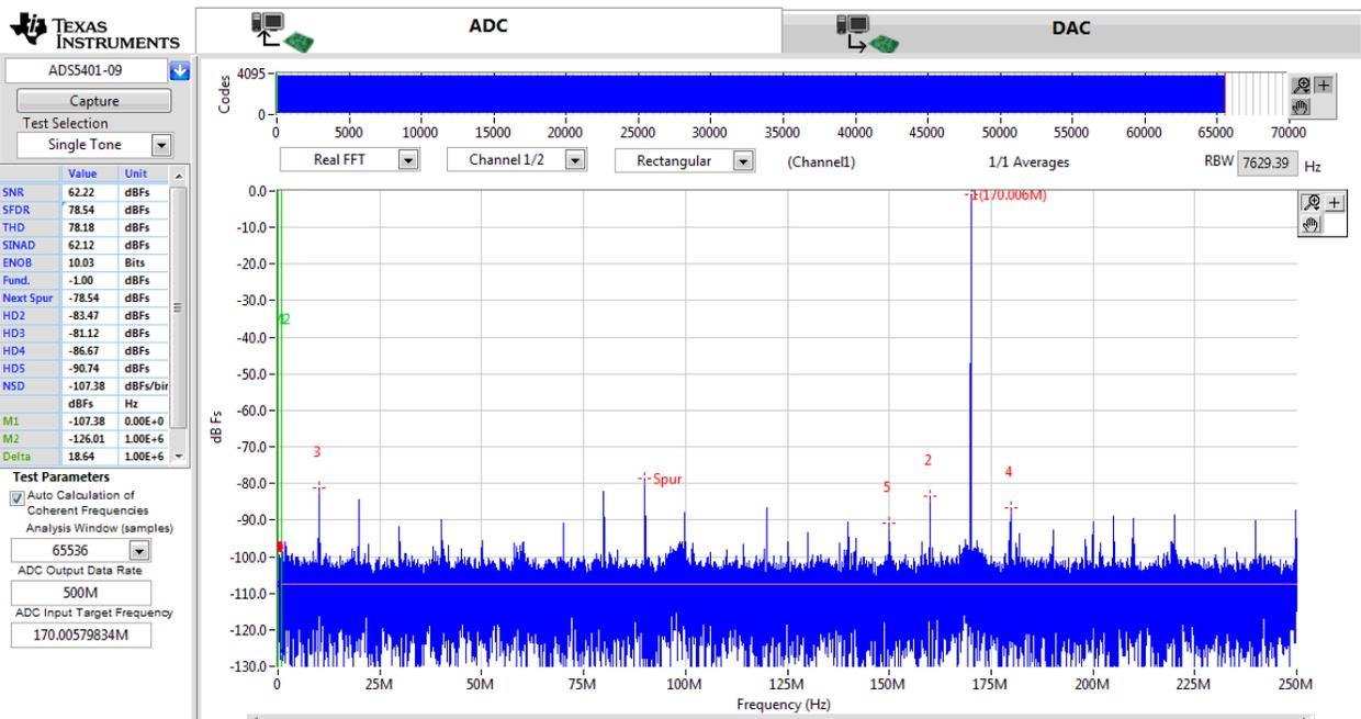
Figure A-4. ADS5407 powered with SMPs and 170-MHz signal frequency
