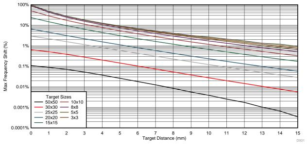
Figure 9. % Maximum Frequency Shift vs Target Distance (in mm)
