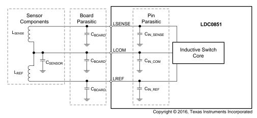
Figure 16. Sensor Capacitance
