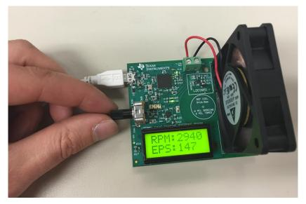
Figure 3. TIDA-00851-LDC0851 Powered by USB Connection
