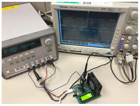
Figure 18. Verification With Hall-Effect-Based Tachometer
