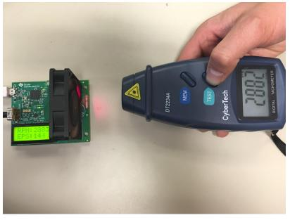
Figure 17. Verification With Optical Tachometer
