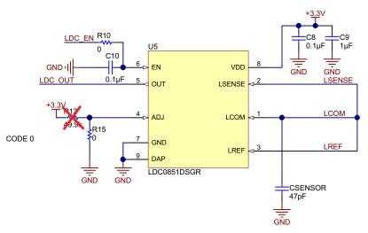
Figure 21. LDC0851 and Sensor Schematics (1)
