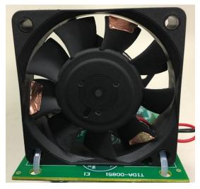
Figure 4. Three Fan Blades Coated With Conductive Material (Copper Tape)
