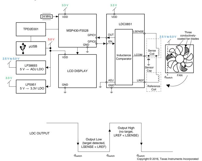
Figure 2. TIDA-00851-LDC0851 System Block Diagram
