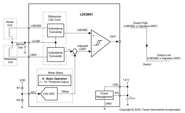
Figure 7. LDC0851 Functional Block Diagram
