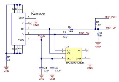
Figure 22. Micro USB Connector and ESD Protection Schematics
