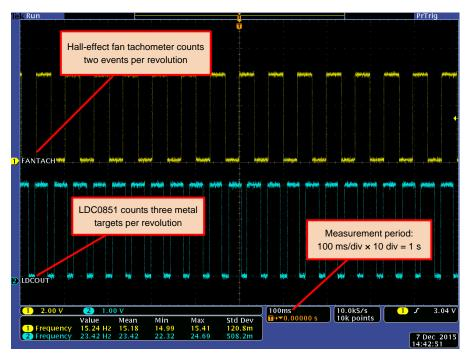
Figure 19. 460 RPM (23 Events per Second) With Hall-Effect Based Verification
