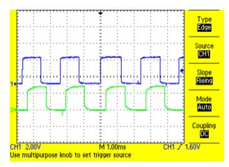
Figure 4. Encoder Phase Offset
