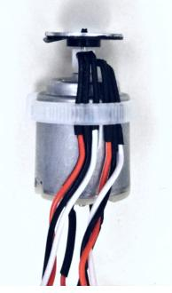
Figure 3. Encoder Setup
