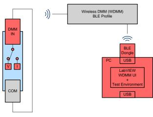
Figure 55. Voltage Resolution Test Configuration
