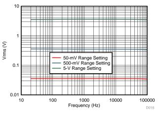
Figure 75. AC Voltage Frequency Response (5-V, 500-mV, 50-mV Sine Wave With 0-V DC Offset)
