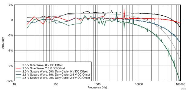
Figure 72. AC Voltage Frequency Response (5-V Range)
