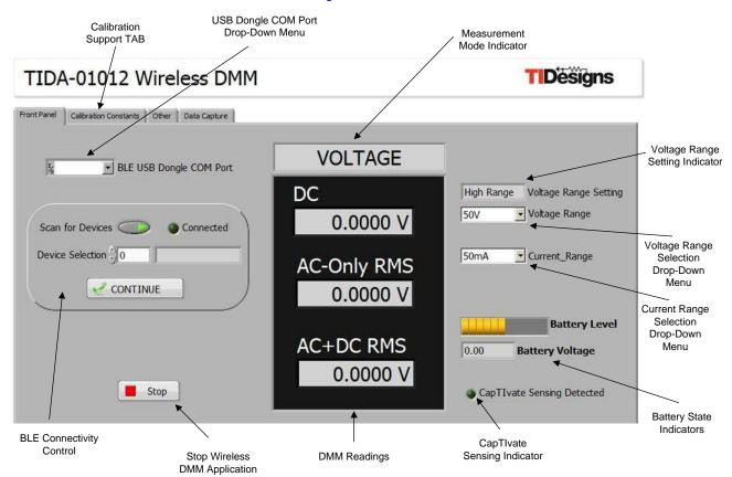
Figure 54. LabVIEW Host Environment Features
