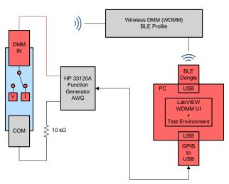
Figure 76. AC Current Frequency Response Test Configuration
