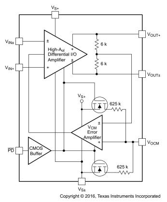
Figure 11. THS4531 Functional Block Diagram
