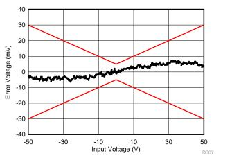
Figure 64. Linearity Plot (50-V Range)
