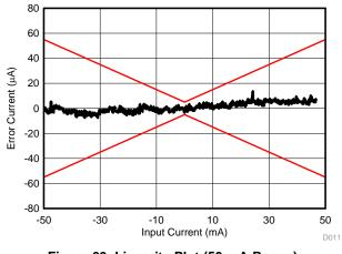
Figure 69. Linearity Plot (50-mA Range)
