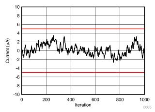
Figure 61. Noise Floor (50-mA Range, 0-V Input)
