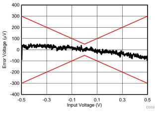
Figure 66. Linearity Plot (500-mV Range)
