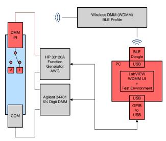
Figure 68. Current Accuracy and Linearity Test Configuration
