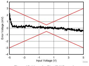
Figure 65. Linearity Plot (5-V Range)
