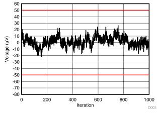
Figure 58. Noise Floor, DC Voltage Mode (500-mV Range, 0-V Input)
