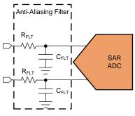
Figure 27. Anti-Aliasing Filter
