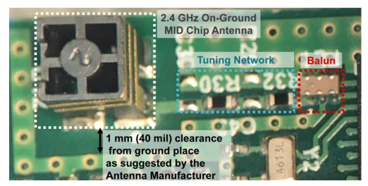
Figure 39. Tuning Network PCB Image
