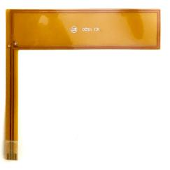
Figure 44. NFC Flex PCB Antenna
