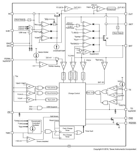
Figure 6. bq24232 Functional Block Diagram
