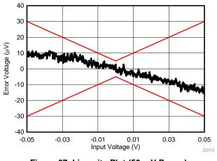
Figure 67. Linearity Plot (50-mV Range)
