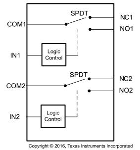
Figure 15. TS3A24159 Functional Block Diagram
