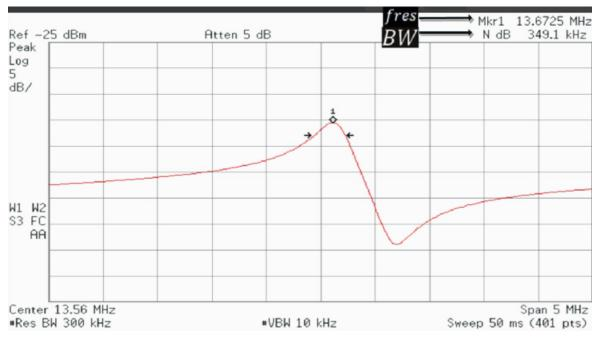
Figure 47. Example of Resonance Curve
