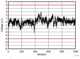
Figure 59. Noise Floor, DC Voltage Mode (50-mV Range, 0-V Input)
