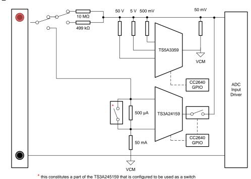
Figure 22. Simplified DMM Front-End Block Diagram
