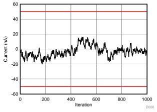
Figure 62. Noise Floor (500-µA Range, 0-V Input)
