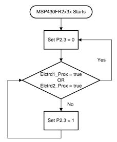
Figure 40. CapTIvate Wake-up Feature Flow Chart
