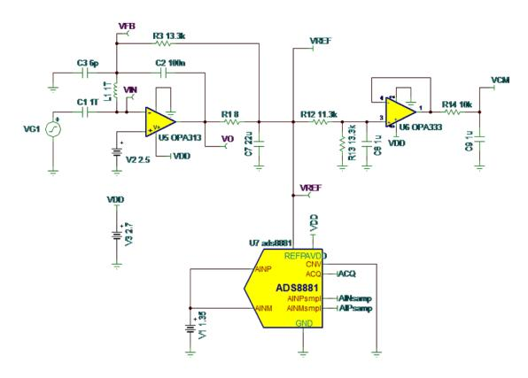
Figure 33. TINA-TI Dual R<sub>ISO</sub> Simulation Schematic
