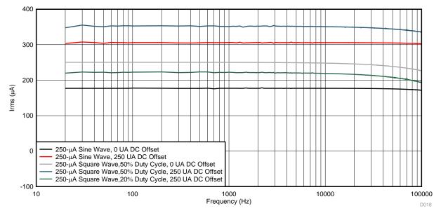
Figure 78. AC Current Frequency Response (500-µA Range)
