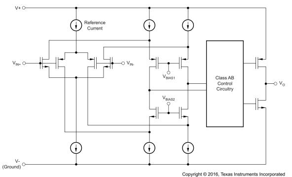
Figure 13. OPAx313 Simplified Schematic
