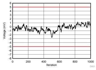
Figure 56. Noise Floor, DC Voltage Mode (50-V Range, 0-V Input)
