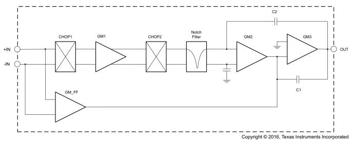
Figure 12. OPAx333 Functional Block Diagram
