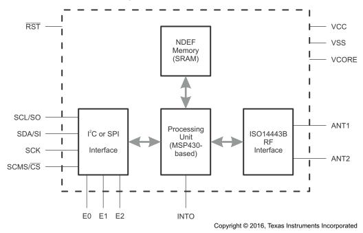
Figure 4. RF430CL330H Functional Block Diagram
