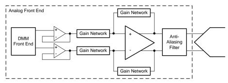
Figure 24. Input Buffer and Gain Network Block Diagram
