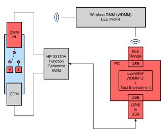
Figure 71. AC Voltage Frequency Response Test Configuration
