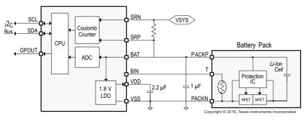
Figure 7. bq27426 Functional Block Diagram
