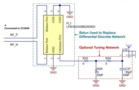
Figure 38. CC2640 Antenna Tuning Network
