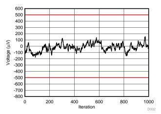
Figure 57. Noise Floor, DC Voltage Mode (5-V Range, 0-V Input)
