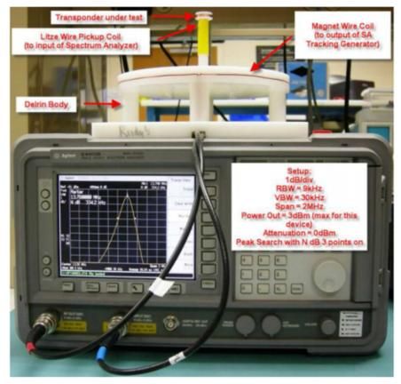
Figure 46. Spectrum Analyzer Tracking Generator
