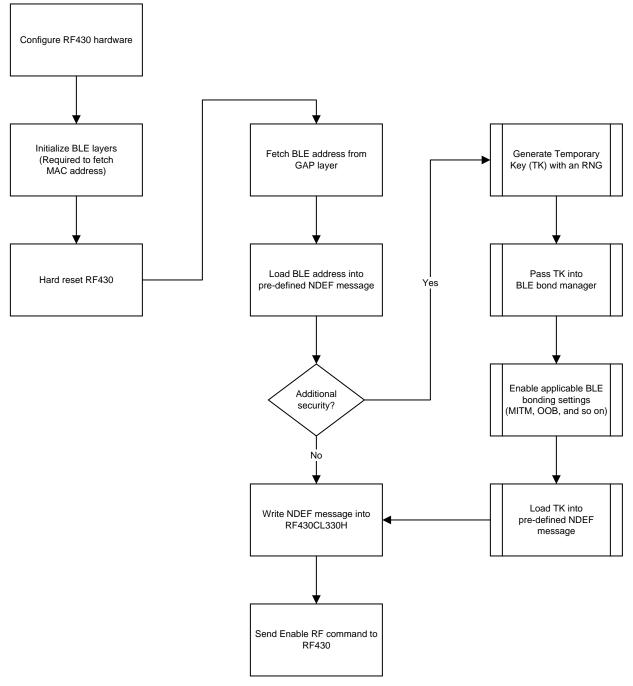
Figure 48. Bluetooth Low Energy Pairing Sequence Flow Chart
