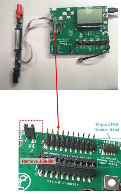
Figure 53. SmartRF06 Evaluation Board for Programming and Debugging
