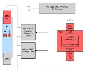
Figure 63. Voltage Accuracy and Linearity Test Configuration
