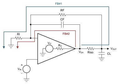
Figure 30. RISO Dual Feedback Configuration for Stability
