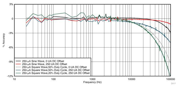
Figure 77. AC Current Frequency Response (500-µA Range)
