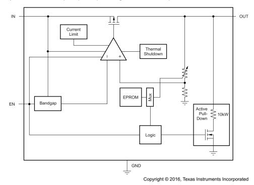
Figure 9. TPS782xx Functional Block Diagram
