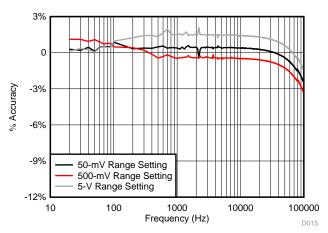
Figure 74. AC Voltage Frequency Response (5-V, 500-mV, 50-mV Sine Wave With 0-V DC Offset)
