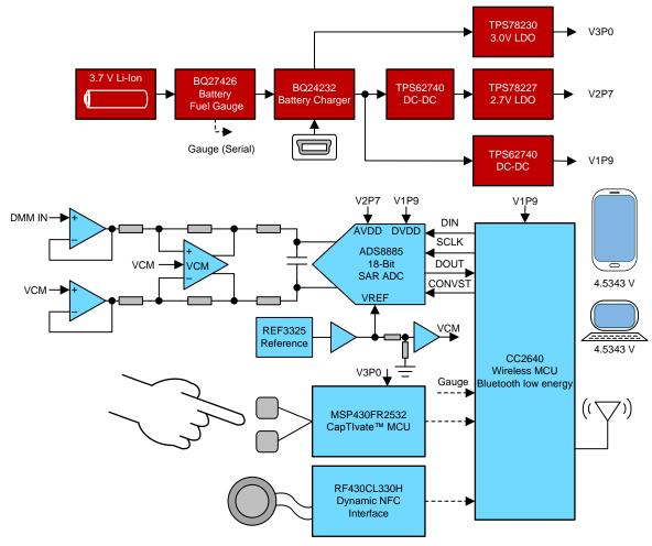
Figure 1. TIDA-01012 Block Diagram
