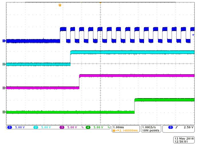
Figure 7. PWM Turnon Timing in Tail Mode
