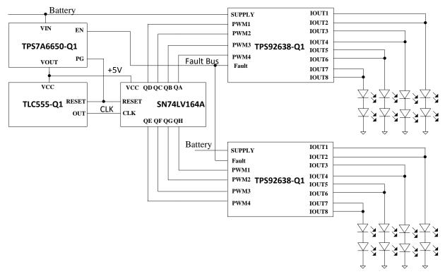
Figure 1. TIDA-01007 System Block Diagram
