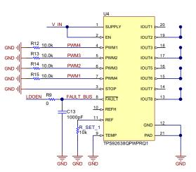
Figure 5. Low  $I_{q}$  of Fault Mode
