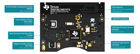
Figure 7. BLE SensorTag Internals (CC2650 Along With Sensors)
