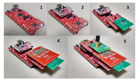
Figure 24. Connecting All Hardware Components of the Gateway
