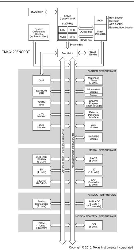
Figure 2. TM4C1294ECPDT MCU High-Level Block Diagram
