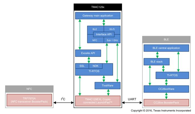
Figure 20. BLE Node Software Architecture Design
