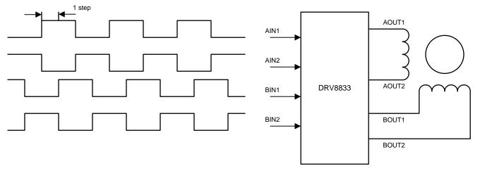
Figure 10. Driving the Stepper Motor in Full-Step Mode
