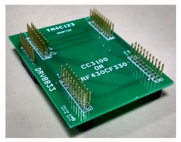
Figure 9. TM4C123 Swizzle Adapter Board
