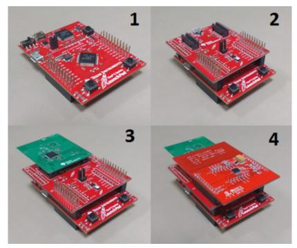
Figure 28. Connecting All Hardware Components of the BLE Node
