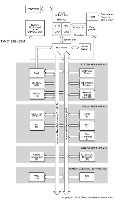
Figure 1. TM4C123GH6PM MCU High-Level Block Diagram
