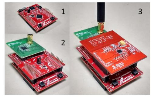
Figure 29. Connecting All Hardware Components of the Sub-1GHz Node
