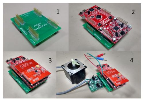
Figure 26. Connecting all Hardware Components of the Wi-Fi Node
