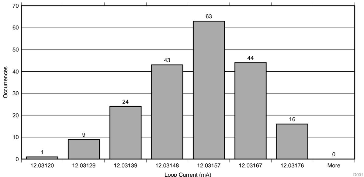
Figure 9. Histogram 32-bit ADC With Internal Reference
