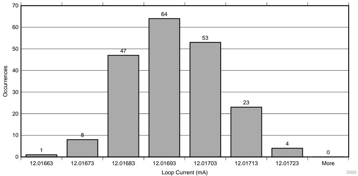
Figure 8. Histogram 32-bit ADC With External Reference
