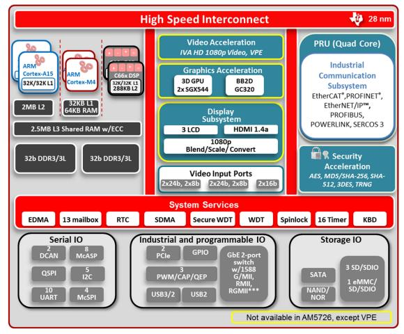
Figure 2. AM572x Block Diagram
