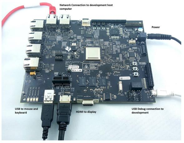
Figure 4. AM572x IDK Setup
