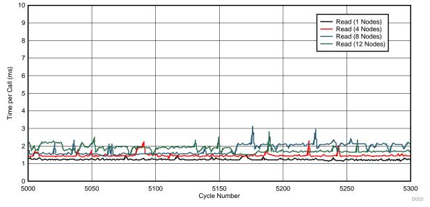
Figure 13. Client Read Call (Non-Registered Node ID)
