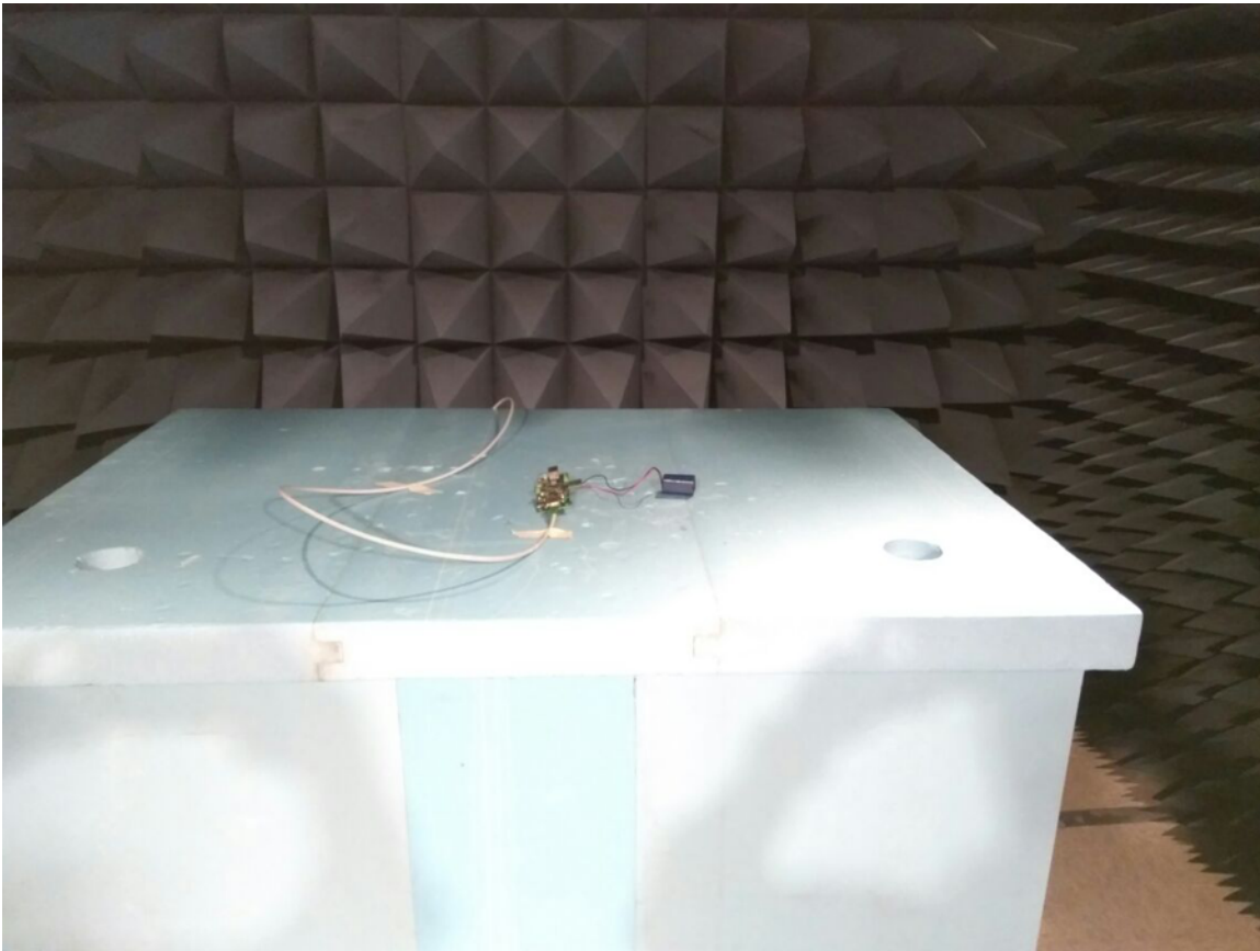
Figure 25. Ethernet PHY + Controller During Radiated Emission Test
