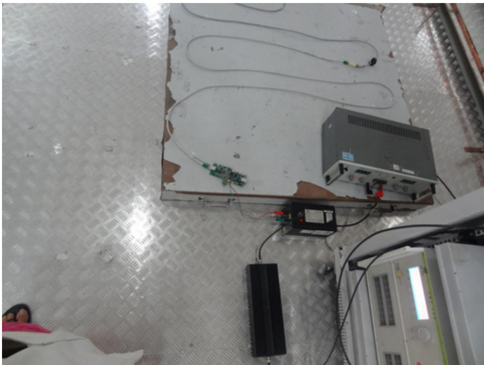
Figure 23. TIDA-00928 Board Testing on Communication Cable With CDN
